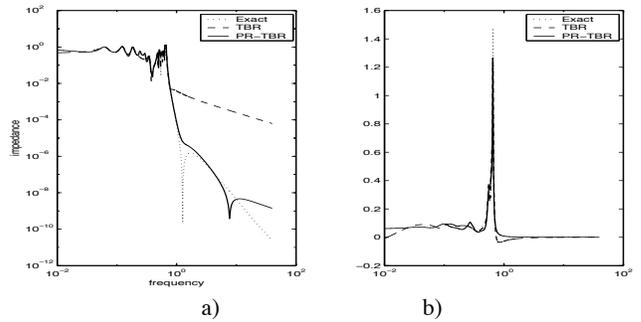
**Figure 3: Left: Magnitude of  $Y_{12}$  for LC line. Right: Minimum eigenvalue of symmetric part of reduced model transfer function. Note that the minimum eigenvalue the TBR model drops below zero for some frequencies, indicating non-passivity.**
