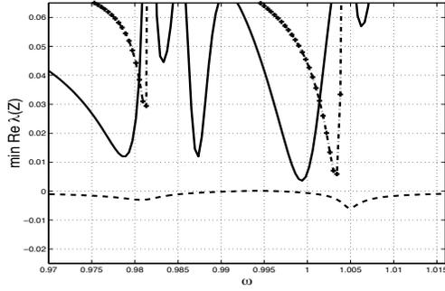
**Figure 1: Minimum eigenvalue of transfer functions used to illustrate non-positive-real reduced model generated by standard TBR procedure. Solid line shows original (positive-real) order-26 transfer function, dashed line shows TBR result of order 7, dashed-dot line shows PR-TBR result of order 7. Note negative sign of TBR results indicating non-positive-realness.**
