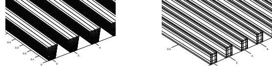
Fig. 5. Structural view of an array of 8 conductors with (a). trapezoidal cross-sections and (b). rectangular cross-sections.
