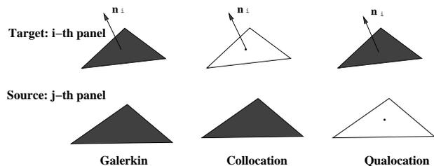
Figure 2: Different discretization configurations
