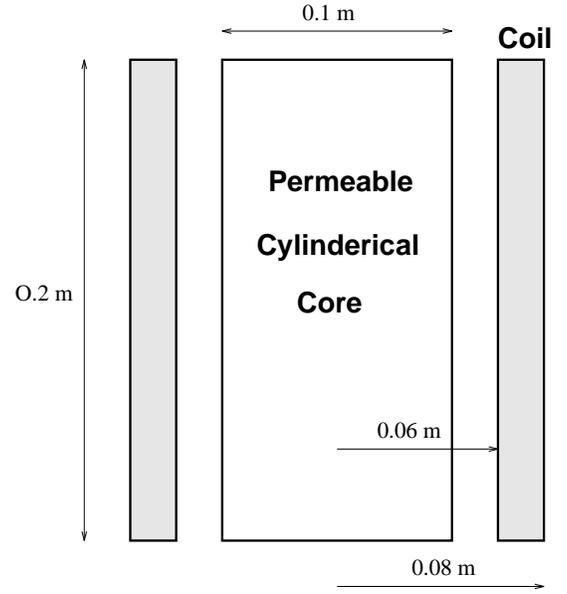
Figure 5: Permeable cylinder and excitation coil.
