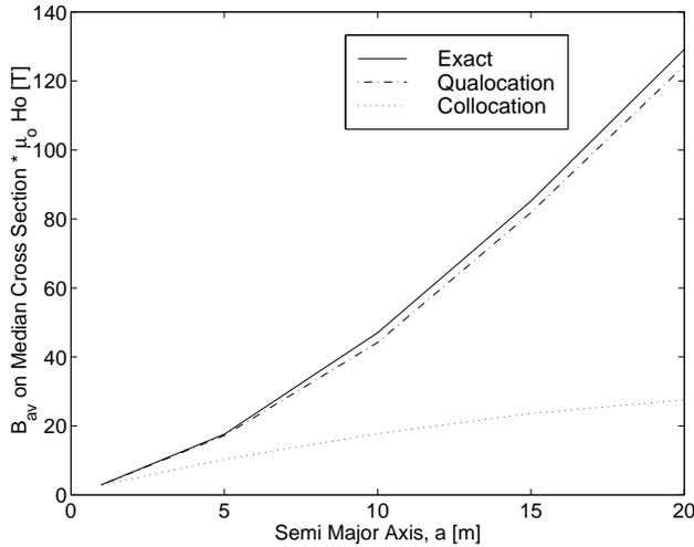
Figure 4: Average flux density over the ellipsoid's median cross section, shown in figure 3, for both collocation and qualocation.
