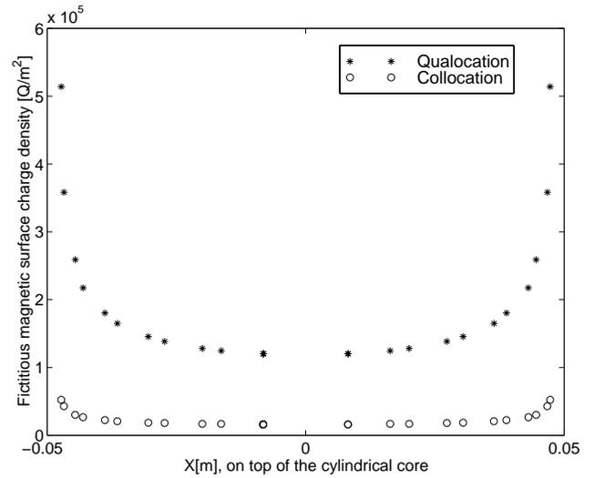
Figure 8: Fictitious magnetic surface charge on cylinder top.
