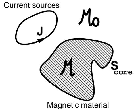
Figure 1: Current sources are outside the magnetic material.
