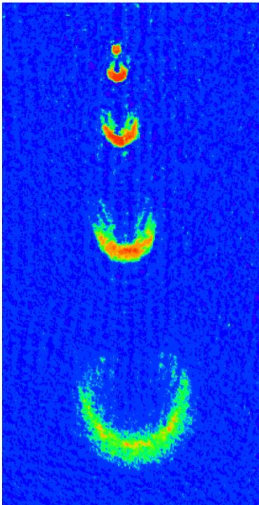
Figure 2: A pulsed atom laser in operation. The picture (field of view 2.5 mm x 5.0 mm) shows pulses of coherent sodium atoms coupled out from a Bose-Einstein condensate confined in a magnetic trap. Every five milliseconds, a short rf pulse rotated the magnetic moment of the trapped atoms, transferring a fraction of these atoms into a quantum state which is no longer confined. These atoms were accelerated downward by gravity and spread out. The atom pulses
