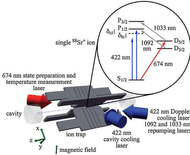
FIG. 1 (color online). Schematic of the experimental setup. A single  $^{88}\text{Sr}^+$  ion is confined in the center of a linear RF Paul trap and coupled to an optical resonator oriented along the trap axis. The inset shows the ion energy levels (solid lines) and the cavity resonance (dashed line).
