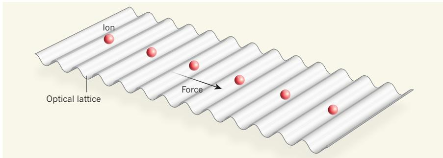
**Figure 1 | Ion chain trapped in a lattice.** Bylinskii *et al.*<sup>2</sup> and Gangloff *et al.*<sup>3</sup> investigate the friction that arises when one or a few ions are forced to slide across optical lattices in which a corrugated energy potential is created by counter-propagating lasers. These simple experiments have provided benchmark tests of long-standing frictional models for sliding crystal surfaces. (Adapted from ref. 2.)
