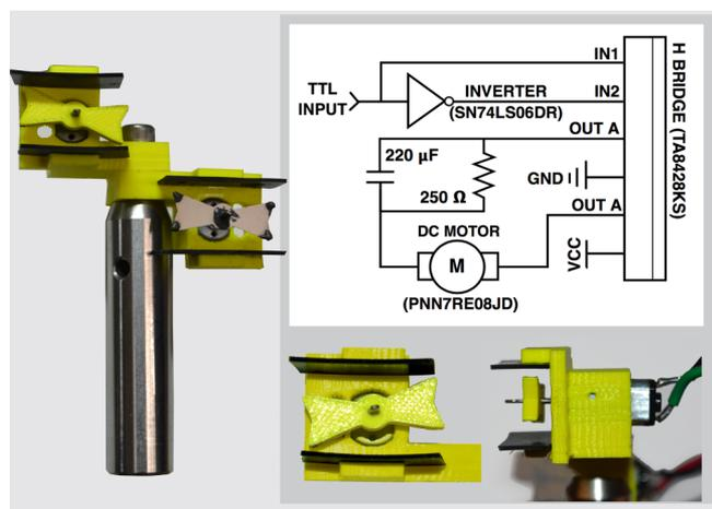
FIG. 2. Shutter units stacked on an optical post (left), side view of shutter with plastic blade (bottom right), and the circuit schematic for a single shutter driving circuit, with part numbers indicated (top right).
