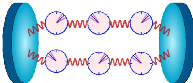
The figure shows how distant atoms, operating as atomic clocks, can be coaxed into a collective state where their dials are correlated: For each clock being ahead when measured there is a clock being behind. The average reading of all clocks is more precise than if the clocks were not correlated. Light is used to synchronize the atoms, creating a kind of superatom which measures time more accurately than independent atoms.
