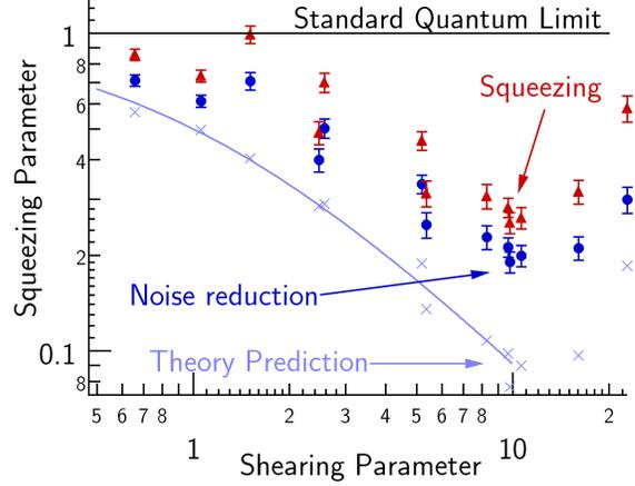
Fig. 7. Shown in blue circles are the variance of  $S_z$  measurements for squeezed states prepared by dynamical evolution. When the loss of contrast is taken into account, we obtain the squeezing values shown as red triangles. The pale blue crosses are estimates of the intrinsic variance of the squeezed states, after subtracting out noise due to imperfect readout; they agree with a simple analytical model [19] over a decade in strength of the shearing interaction.
