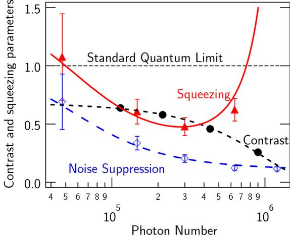
Fig. 6. Measurement-based squeezing: as more and more photons are used for the measurement of  $S_z$ , the noise on the  $S_z$  component of the state is reduced. However the coherence of the resulting state is also reduced by inhomogeneous light phase shifts (black). Balancing the reduction of noise against the loss of signal gives the improvement in angular resolution for the collective spin (squeezing, red).
