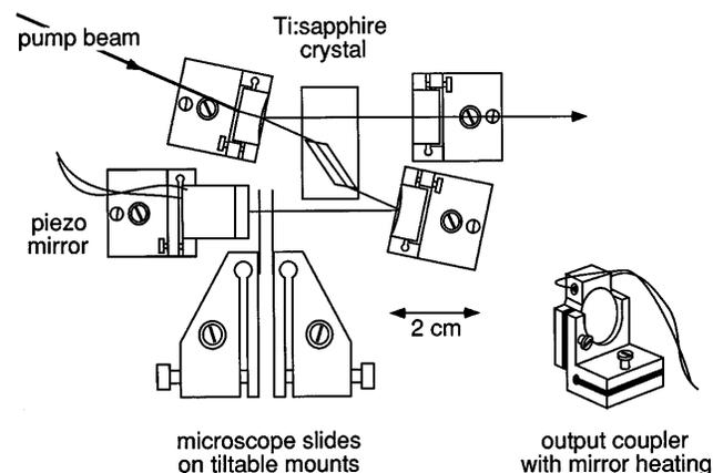
Fig. 1. Mechanical design for a compact tunable Ti:sapphire laser.
