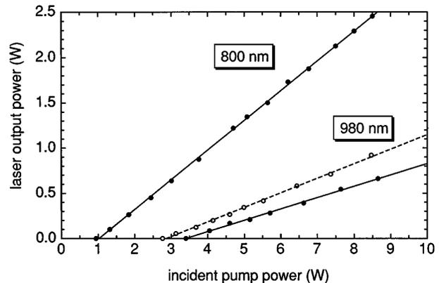
Fig. 2. Laser output versus pump power incident upon the curved resonator mirror. The dashed line describes the laser at 980 nm when the glass plate étalons are removed from the cavity.
