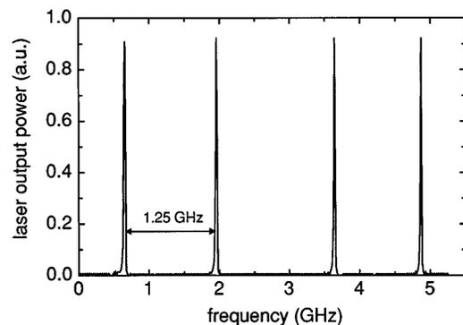
Fig. 3. Laser output spectrum recorded with a Fabry-Perot spectrum analyzer (free spectral range 3 GHz). The two modes are separated by the free spectral range of the laser cavity (1.25 GHz). The observed linewidth of 3 MHz is limited by the resolution of the spectrum analyzer.
