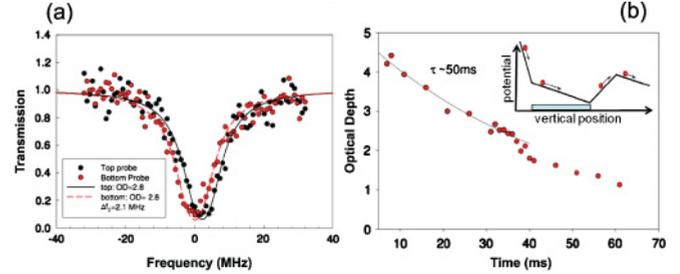
FIG. 8. (Color online) Atoms inside the fiber. (a) Doppler shift of the falling atom cloud observed by using two probes propagating through the fiber in opposite directions. (b) Lifetime of the atoms inside the fiber. Inset: A qualitative sketch of the potential along the fiber axis experienced by the atoms as they load into the fiber-guided dipole trap.
