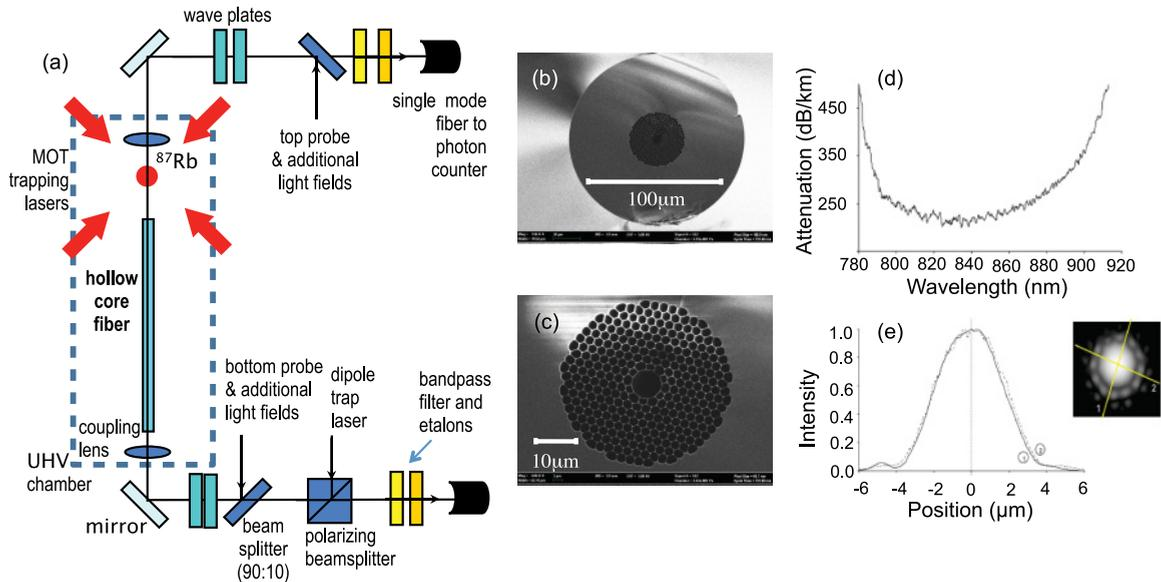
FIG. 1. (Color online) (a) The schematics of the experimental setup. (b) Scanning electron microscope (SEM) image of a cleaved hollow-core photonic-crystal fiber, Model HC-800-02, from Blaze Photonics. (c) Detail of the photonic-crystal region with the hollow core in the center. Manufacturer's specifications for (d) losses of guided mode propagating in the fiber as a function of wavelength and (e) near-field intensity distribution of the guided mode.
