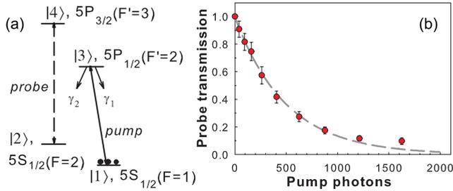
FIG. 7. (Color online) (a) Calibration of the number of atoms inside the fiber by counting the number of photons required to transfer the amount of atoms required to cause  $\mathcal{D}^{\text{opt}} = 1$  on a given probe transition. (b) With  $\gamma_1 \approx \gamma_2$ , fitting an exponential (dashed line) to the measured data (red dots with error bars) yields  $\eta \approx 0.42$  as the value of the prefactor from Eq. (3).
