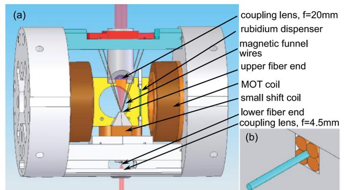
FIG. 2. (Color online) (a) Fiber assembly. (b) The anchoring of the fiber inside the mount.
