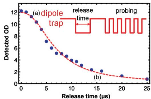
FIG. 9. (Color online) Temperature estimate from a TOF measurement. (a) The time sequence diagram: After the atoms are released from the trap and then recaptured, the trap is modulated for the  $D^{\text{opt}}$  measurement. (b) Optical depth of the recaptured cloud as a function of the release time. The dashed red line represents a fit based on the Gaussian cloud expansion model.
