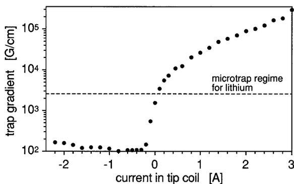
FIG. 4. Calculated magnetic field gradient of the trap for various currents of the tip coil. The current in the counter coil is set to a fixed value of 2.6 A.
