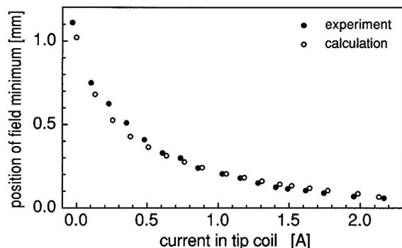
FIG. 3. Observed position (solid dots) of the trap center for various currents in the tip coil as compared to the results of the numerical calculation (white dots). The current in the counter coil is set to a fixed value of 2.6 A. The experimental errors are smaller than the size of the dots.
