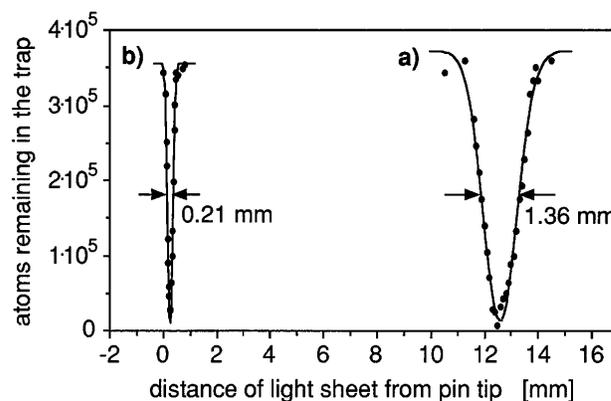
FIG. 2. Observed shape of the atomic cloud (a) in the shallow field after loading from a magneto-optical trap and (b) after compression in the steep potential of the  $\mu$  tip trap at a current in the tip coil of 1.2 A.
