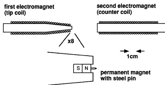
FIG. 1. Setup of the  $\mu$  tip trap. A sharp steel pin is magnetized by a permanent magnet and exposed to a variable magnetic field that is generated by two electromagnets.
