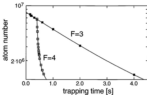
FIG. 2. Decay of the trapped gas for different hyperfine ground states. The open squares show the atom number upon preparation in the upper hyperfine state at the time  $t_0 = 400$  ms. The initial density is  $1.1 \times 10^{12} \text{ cm}^{-3}$ . The solid lines are fits including a two-body loss.
