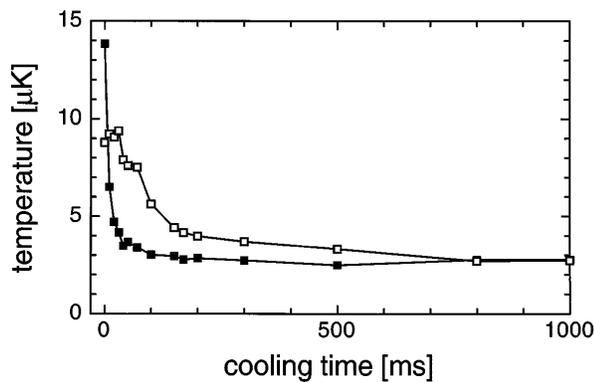
FIG. 4. Evolution of the axial (solid squares) and radial (open squares) temperatures. The degenerate Raman sideband cooling is applied only along the steep axial direction.
