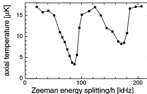
FIG. 3. Axial temperature after 200 ms of degenerate Raman sideband cooling as a function of the Zeeman energy difference between  $m = 2$  and  $m = 3$ .
