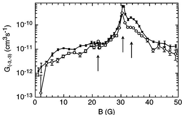
FIG. 2. The two-body loss rate coefficient for the state  $F = 3$ ,  $m_F = -3$  as a function of magnetic field for  $14 \mu\text{K}$  (open circles) and  $4 \mu\text{K}$  (solid squares). A strong resonance occurs at 31 G, a weaker one at 34 G, and possibly another at 22 G.
