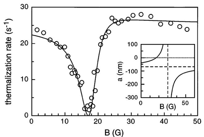
FIG. 1. The thermalization rate for the state  $F = 3, m_F = 3$  between the axial and radial motions as a function of magnetic field for a temperature of 9  $\mu\text{K}$  and a mean density of  $1.5 \times 10^{11} \text{ cm}^{-3}$ . The solid line is a fit assuming a simple dispersive shape for the scattering length. The inset shows the scattering length as calculated from the best-fit parameters. The scattering length is positive between 17 and 30 G.
