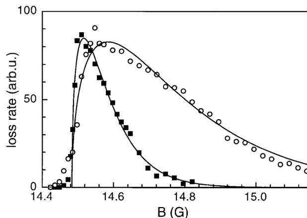
FIG. 3. Expanded view of the narrow loss peak near 14.48 G for  $3.3 \mu\text{K}$  (solid squares) and  $8 \mu\text{K}$  (open circles) with fitted Boltzmann distributions. The sharp temperature-independent left edge indicates a linewidth of  $2\pi \times 5$  kHz.
