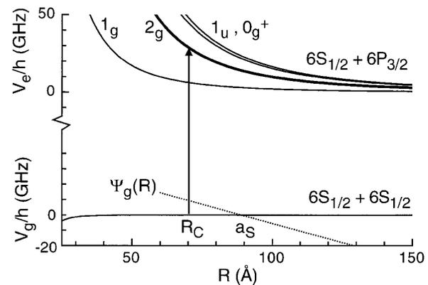
FIG. 1. Ground state and repulsive excited state potentials for the  $\text{Cs}_2$  molecule. The blue detuned light is resonant with the potential difference at the Condon point  $R_C$ . Also shown is a ground state wave function in the low-energy limit for positive scattering length  $a_s$ . The radiative loss is minimized when the node of the scattering wave function is tuned to the Condon point.
