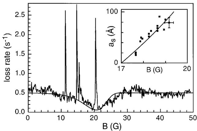
FIG. 2. Radiative loss rate for a detuning of  $2\pi \times 32$  GHz and an average intensity of  $26 \text{ mW/cm}^2$ . The gas temperature and peak density are  $5.0 \mu\text{K}$  and  $3 \times 10^{12} \text{ cm}^{-3}$ , respectively. The broad feature corresponds to the suppression of light-assisted collisions when  $a_s$  is positive and close to the Condon point  $R_C$ . Superimposed are very narrow resonances with high radiative loss.
