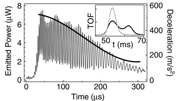
FIG. 4. The emitted power (thin line) during the illumination of a falling atomic cloud. The beat frequency is used to calculate the deceleration (thick line). The inset shows the time-of-flight signal, in arbitrary units, of atomic clouds without (gray line) and with (black line) a  $400 \mu\text{s}$  exposure to the pump beam. Here the pump  $I/I_s = 420$ ,  $\delta_a/2\pi = -1.580$  GHz, and  $\Delta_c/2\pi = -10$  MHz. The atom number is  $N = 2.6 \times 10^7$ .
