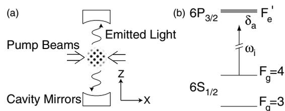
FIG. 1. (a) Schematic experimental setup. Atoms falling along the cavity axis are illuminated by horizontal pump beams and self-organize into a density grating, emitting into the cavity. (b) Cs  $D_2$  line. The atom approximates an open two-level system  $F_g = 4 \rightarrow F_e'$  since the light-atom detuning is much greater than the excited state hyperfine splitting.
