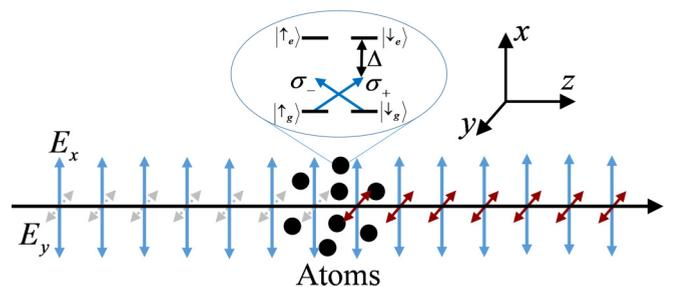
FIG. 5. A coherent pulse propagating in the  $z$  direction interacts off-resonantly with an ensemble of atoms with ground states  $|\uparrow_g\rangle, |\downarrow_g\rangle$  and excited states  $|\uparrow_e\rangle, |\downarrow_e\rangle$ . The  $x$  polarization of the pulse is in a strong coherent state (blue arrow) and the  $y$  polarization is in the vacuum state (gray arrow). The forward-scattered light is in the  $y$  polarization and also propagates along  $z$  (red arrow).
