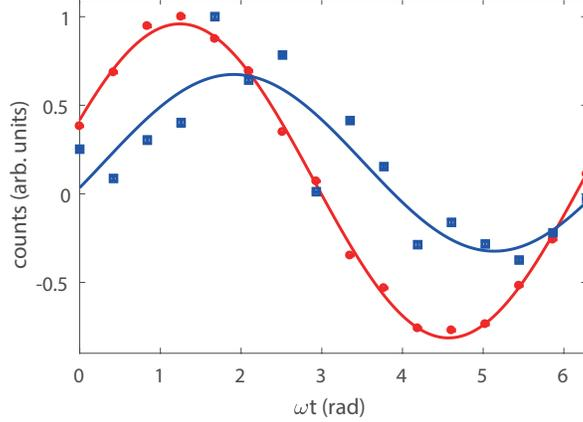
FIG. S1. **Signal phase reconstruction** The signal coherent state is mixed with a 30-MHz-detuned phase reference. By extracting the phase of the beatnote, we reconstruct the phase of the signal state. The red circles and blue squares and the corresponding fitting curves represent the sinusoidal beatnote for the signal state before and after the conditional interaction, respectively.
