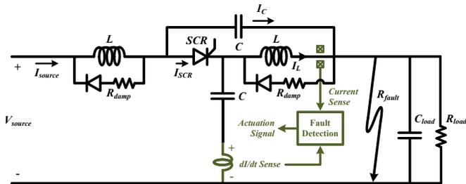
Figure 8. Fault detection sense nodes in a Z-source circuit breaker.
