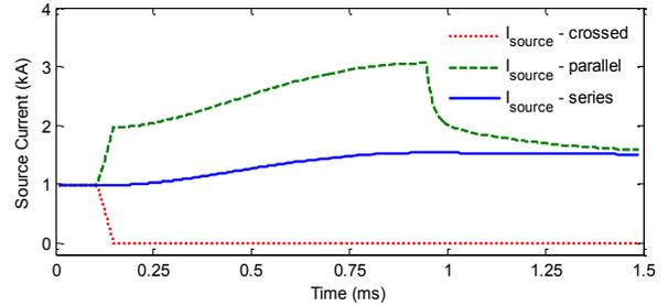
Figure 4. Comparison of the reflected fault current at the source among the three Z-source circuit breaker topologies.
