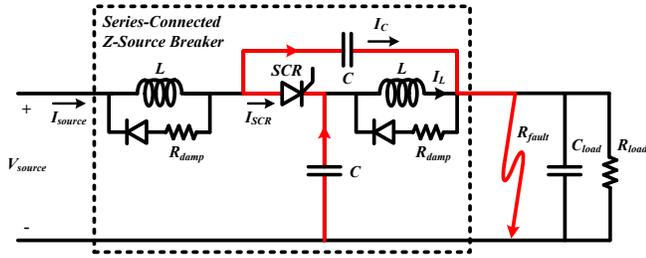
Figure 2. New series-connected Z-source circuit breaker topology.
