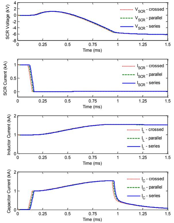
Figure 3. Fault clearing waveforms for the three Z-source circuit breakers. Waveforms for the parallel-connected and series-connected are shifted right by  $10\mu\text{s}$  and  $20\mu\text{s}$  respectively for clarity.
