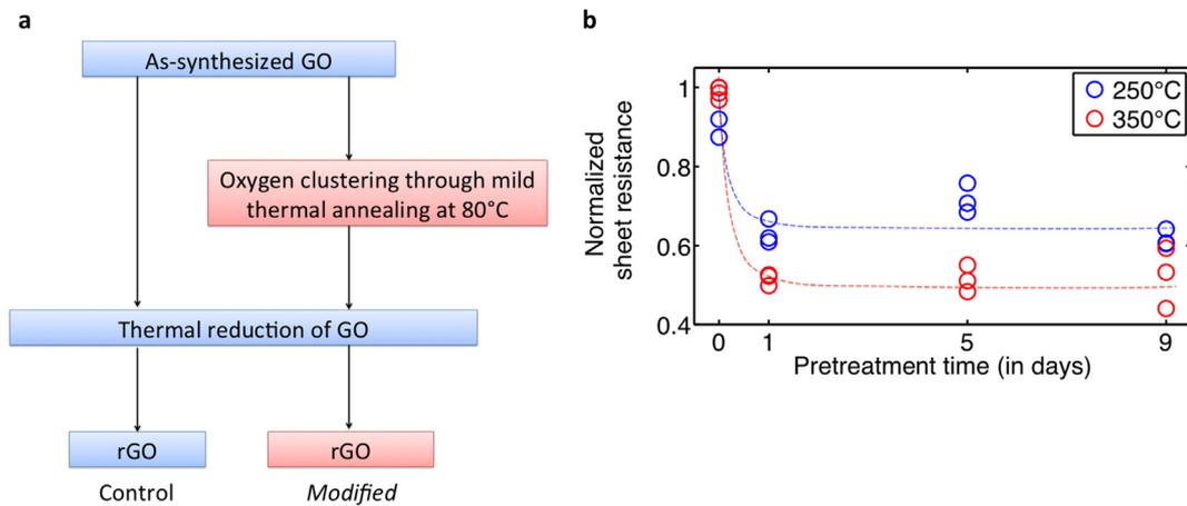
**Fig. 4. Electrical measurements on rGO thin films.** a) Schematic of the experimental procedure employed. b) Sheet resistances of *modified*-rGO thin films (day 1–9) prepared by drop-casting show reduced values compared to that of the control rGO sample (day 0). The trend is represented by the dotted lines and the reduction temperatures are listed. (A color version of this figure can be viewed online.)
