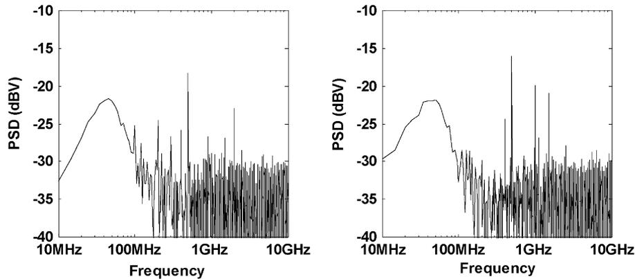
Fig. 13. Measured PSDs of  $V_{dd}$  noise at two different times in the noise period with the links operating at 2 Gb/s.
