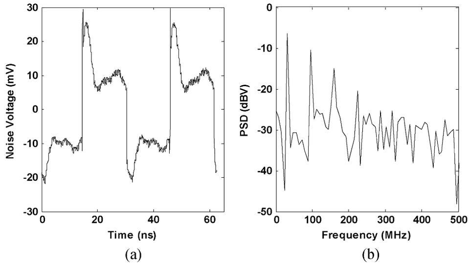
Fig. 9. Measured (a) waveform and (b) PSD of injected 32-MHz square wave on  $V_{dd}$ . The PSD has been scaled by the Nyquist frequency (10 GHz) to calculate the power and shown with the unit (dBV) instead of the usual ( $\text{dB V}^2/\text{Hz}$ ). For PSDs in dBV, the average level in dB corresponds roughly to the noise  $\sigma$ .
