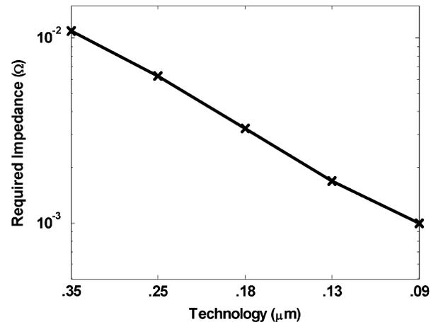
Fig. 1. 10% noise budget required impedance for a 100-W chip across technologies.
