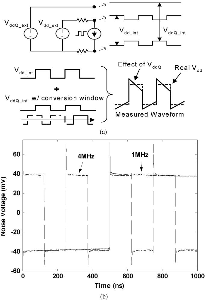
Fig. 8. (a) Potential effect of uncoupled  $V_{\text{ss}}$  noise through  $V_{\text{ddQ}}$  on measured waveform. (b) Measured noise injected on  $V_{\text{ddQ}}$  (mean subtracted) at 1 MHz and 4 MHz with a 500-ns conversion window.
