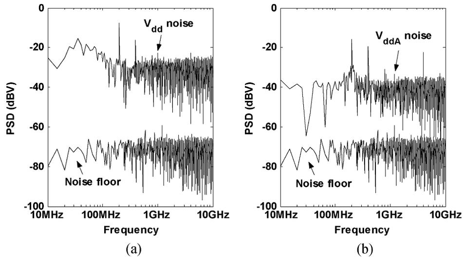
Fig. 12. Measured PSD with the noise floor for (a)  $V_{dd}$  and (b)  $V_{ddA}$ .
