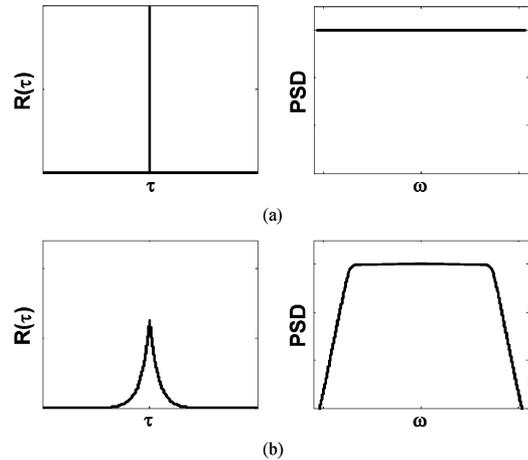
Fig. 2. Autocorrelation and power spectral density for (a) white noise and (b) low-pass filtered white noise.
