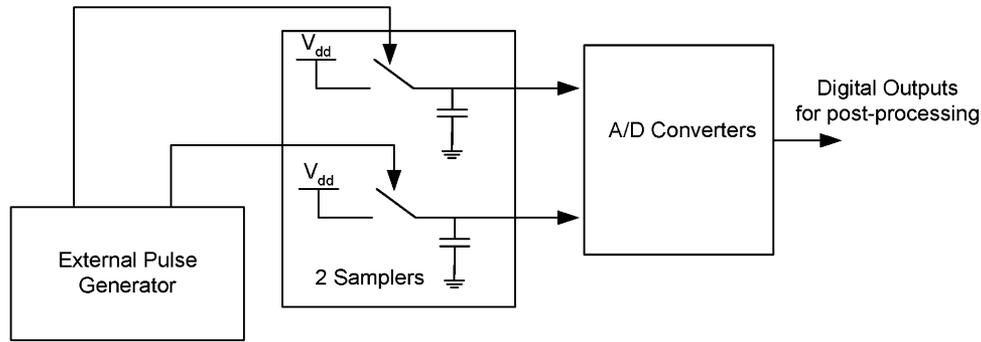
Fig. 4. Supply noise measurement system block diagram.
