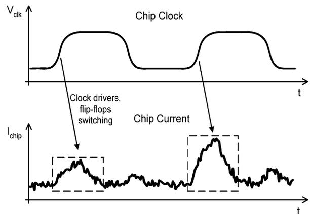
Fig. 3. Example of the clock modulating the chip current consumption waveform.
