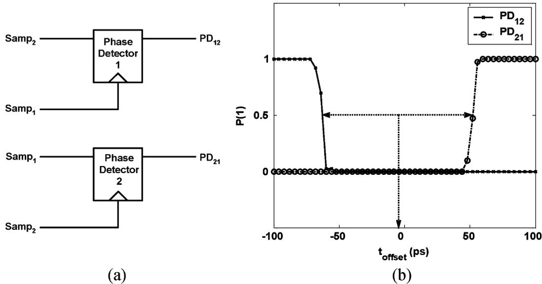
Fig. 7. (a) On-chip flip-flop phase detectors for timing calibration. (b) Measured probability of each phase detector outputting a 1 versus timing offset between  $\text{Samp}_1$  and  $\text{Samp}_2$ . Negative  $t_{\text{offset}}$  indicates  $\text{Samp}_1$  is skewed to arrive after  $\text{Samp}_2$ .
