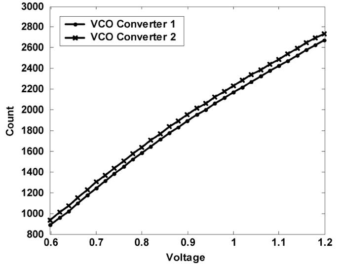
Fig. 6. VCO calibration curves with a 1- $\mu\text{s}$  conversion window.
