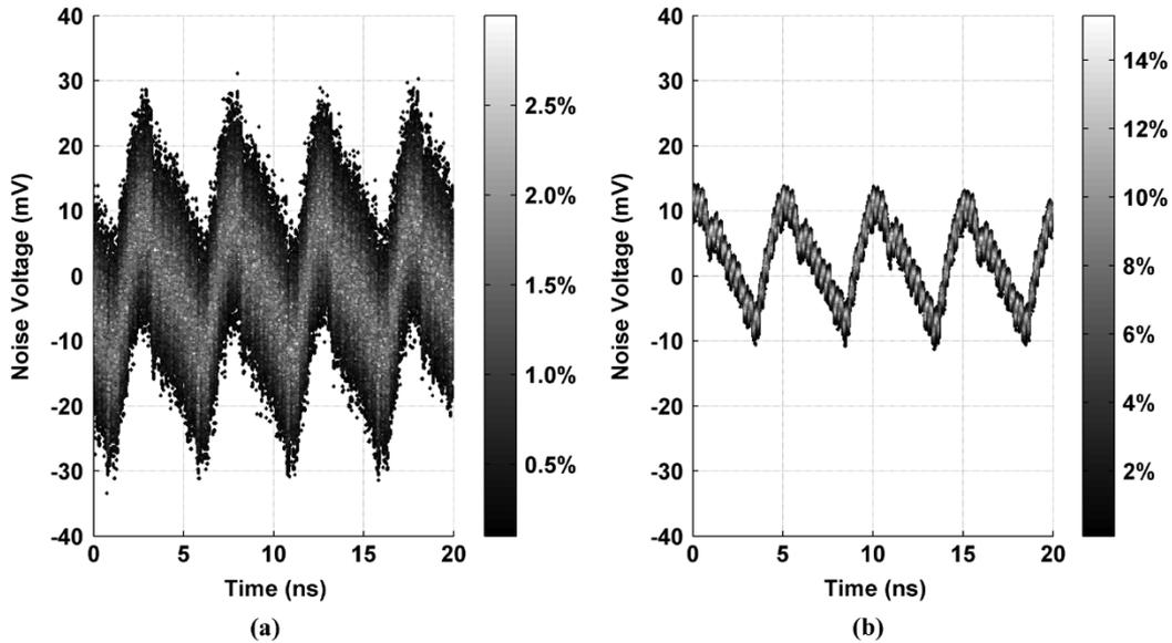
Fig. 10. Measured noise distributions on (a)  $V_{dd}$  (b)  $V_{dda}$ .
