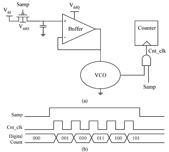
Fig. 5. (a) VCO converter schematic. (b) Example waveforms.
