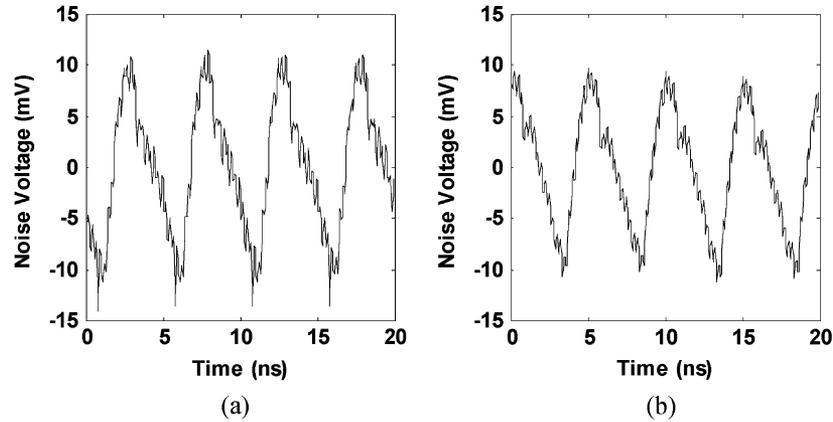
Fig. 11. Measured deterministic noise on (a)  $V_{dd}$  and (b)  $V_{ddA}$ .
