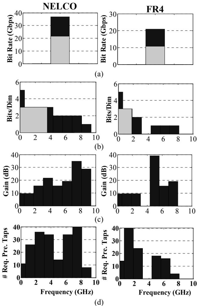
Fig. 5: (a) Total bit rate for MT and BB systems over NELCO (left) and FR4 (right) channels. (b) Bit loading over same channels. (c) Minimum required voltage gain per sub-channel. (d) Minimum number of required precoder taps (real and imaginary, diagonal and cross) per sub-channel.
