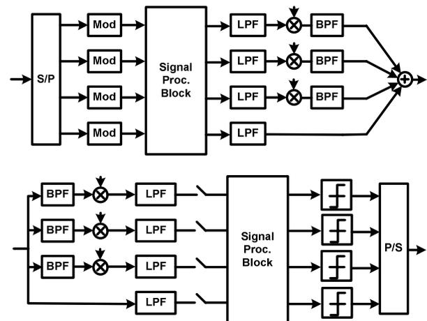
Fig. 2: General block diagram of an AMT transmitter (top) and receiver (bottom). Some blocks might not exist in a specific architecture.
