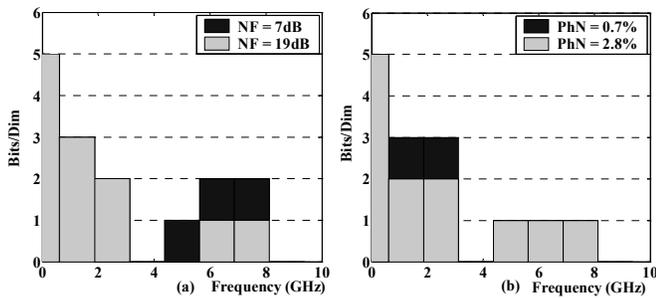
Fig. 6: Bit loadings for MT over FR4 channel when noise figure is changed by  $\pm 6$ dB, phase noise =  $5^\circ$  (a) and when carrier phase noise is changed by a factor of 2, noise figure = 13dB (b).
