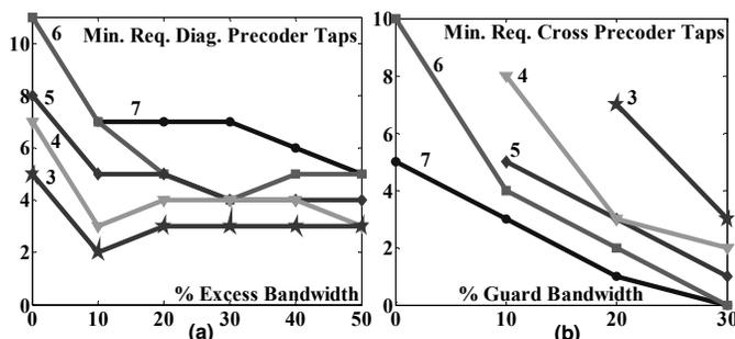
Fig. 4: Minimum number of diagonal equalizer tap per dimension for target performances of 3bits/dimension (a) and Minimum number of cross equalizer taps per dimension per neighbor for target performances of 3bits/dimension, (b). Butterworth filters are used both at the Tx and the Rx and ideal channel is assumed for both figures.
