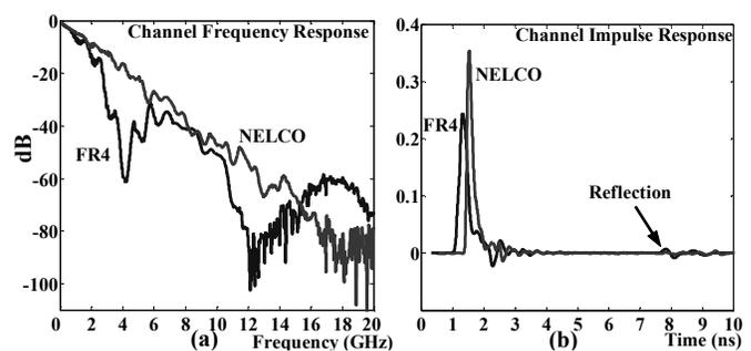
Fig. 1: Frequency Responses (a) and impulse responses (b) of typical link channels. The notches in the frequency response of the FR4 channel and the reflection taps towards the tail of its impulse response are the effects of via stubs.
