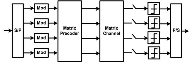
Fig. 3: Baseband equivalent of an AMT system with matrix precoding.
