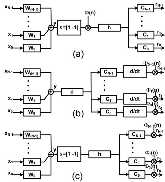
Fig. 5: (a) Transmitter jitter model. (b) Receiver jitter model (c) Alternative receiver jitter model.
