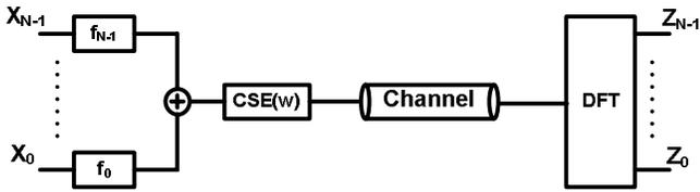
Fig. 2: General DMT architecture with channel shortening filter at the Tx.
