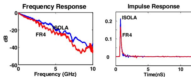
Fig. 1: Left: Frequency responses of sample channels. Right: Their impulse responses. The FR4 channel is the mid-plane 20" FR4 channel considered for IEEE 802.3 and the ISOLA channel is an improved channel with orthogonal line card connections.
