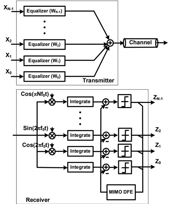
Fig. 3: Analog MT architecture with linear transmit equalization and MIMO DFE.
