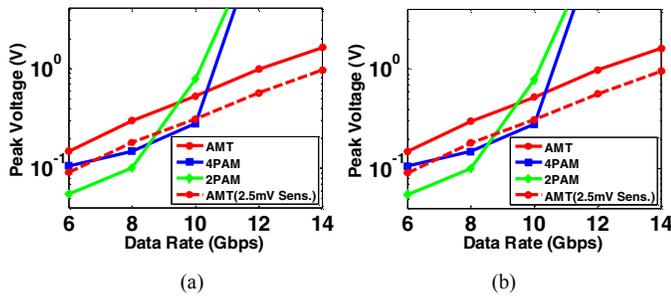
Fig. 6: Minimum required peak voltage over FR4 (a) and ISOLA (b) channels.
