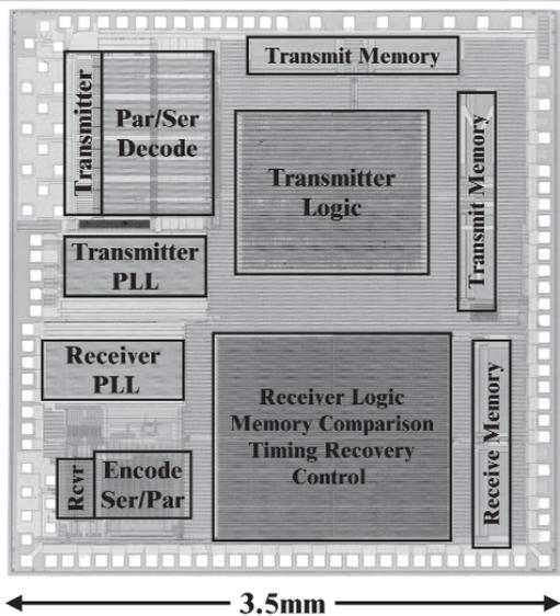
Figure 4.1.7: Chip micrograph.
