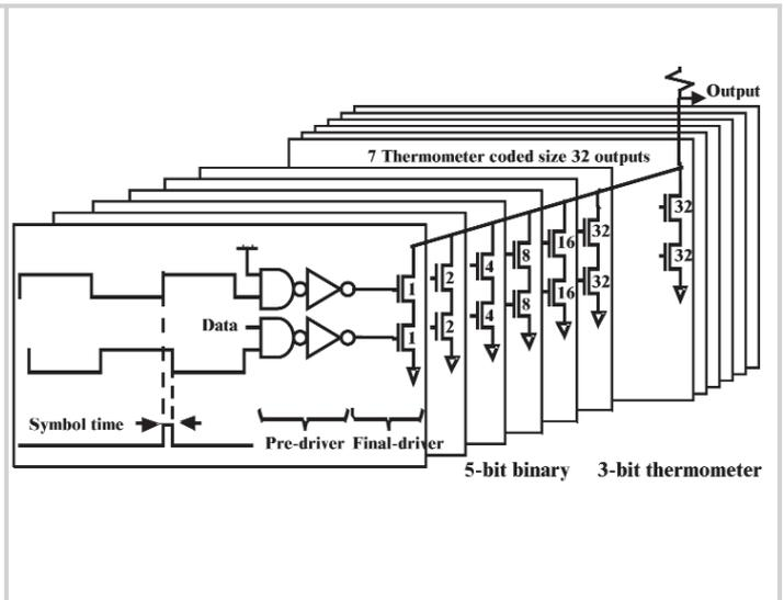
Figure 4.1.2: D/A converter implementation.
