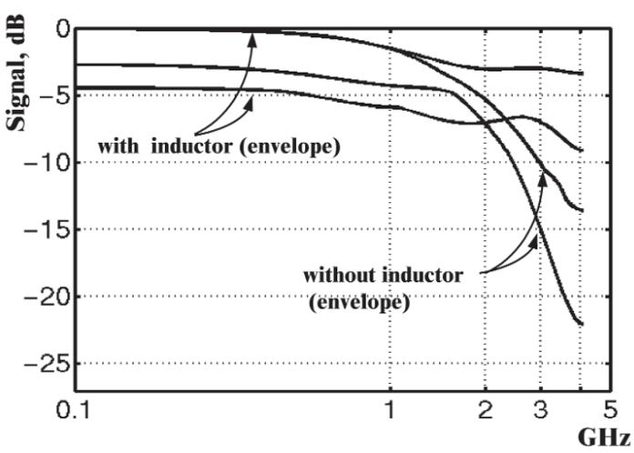
Figure 4.1.5: Transceiver frequency response w/ & w/o inductors.
