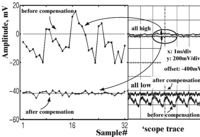
Figure 4.1.3: Transmitter DC coupling.
