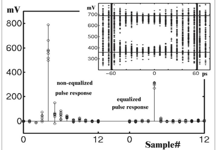
Figure 4.1.6: Transceiver pulse response and equalized eye.
