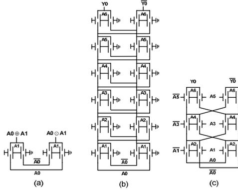
Figure 7. Implementation of (a) a two input XOR/XNOR gate and (b) the  $Y_0$  sub-circuit (c)  $Y_0$  sub-circuit with signals on body terminals
