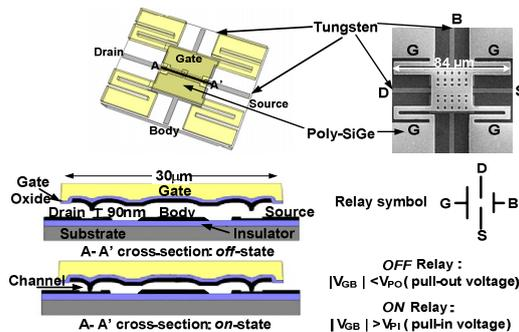
Figure 1. SEM, diagram, circuit symbol and operating states of the current MEM relay device
