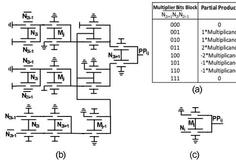
Figure 6. (a) Booth encoding table, (b) Partial product generation circuit for Booth encoded generation, (c) Simple AND gate partial product generation
