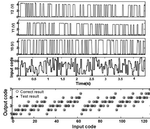
Figure 12. Experimental results of the (7:3) compressor
