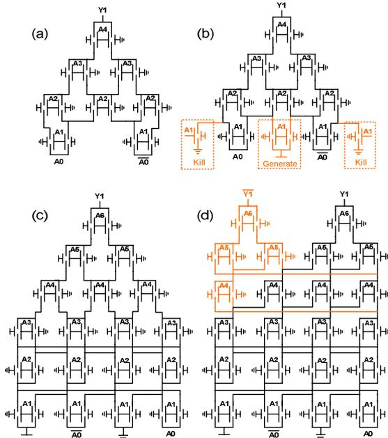
Figure 8. Steps toward implementation of the  $Y_1$  sub-circuit of a complementary (7:3) compressor. (a) propagation paths for  $Y_1$  of the (5:3) compressor, (b)  $Y_1$  the (5:3) compressor, (c)  $Y_1$  of the (7:3) compressor and (d)  $Y_1$  of full complementary (7:3) compressor
