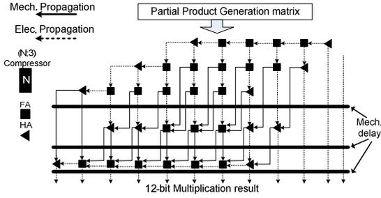
Figure 3. A 6-bit relay multiplier built with full and half adders
