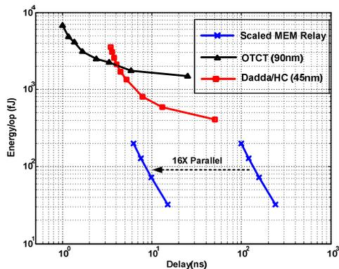
Figure 10. Energy/throughput comparison of CMOS and scaled MEM relay-based 16-bit multipliers
