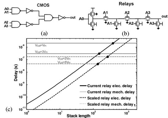
Figure 2. A 4-input AND built with CMOS (a) and MEM-relays (b). Electrical vs. mechanical delay for current (1  $\mu\text{m}$  lithographic process) and scaled (90 nm lithographic process) relays (c)
