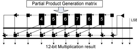
Figure 4. A 6-bit relay multiplier built with (7:3) and smaller compressors
