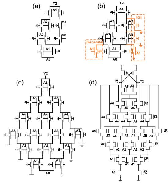
Figure 9. Steps toward implementation of the  $Y_2$  sub-circuit of a (7:3) compressor: (a) propagation paths for  $Y_2$  of the (5:3) compressor, (b)  $Y_2$  of the (5:3) compressor, (c)  $Y_2$  of the (7:3) compressor, (d)  $Y_2$  of the (7:3) CMOS compressor [5]
