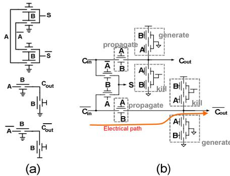
Figure 5. Implementation of (a) half adder and (b) full adder [2]
