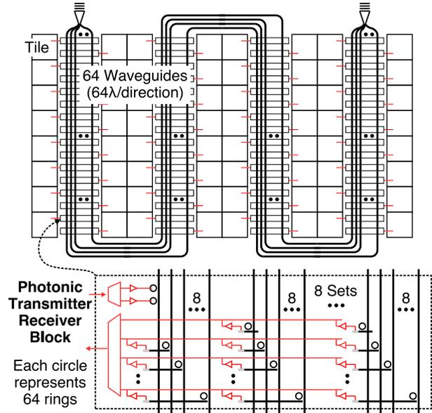
**Figure 5: Serpentine Layout for 64x64 CMXbar** – Electrical circuitry shown in red. 64 waveguides (8 sets of 8) are either routed between columns of tiles (monolithic integration) or over tiles (3D integration). One 128 b/cycle channel is mapped to each waveguide, with  $64 \lambda$  going from left to right and  $64 \lambda$  going from right to left. Each tile modulates a unique channel and every tile can receive from any channel.
