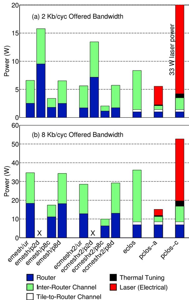
**Figure 12: Dynamic Power Breakdown** – Power of *eclos* and *pclos* did not vary significantly across traffic patterns. (a) LTBw systems at 2 kb/cycle offered bandwidth (except for *emesh/p2d* and *ecmeshx2/p2d* which saturated before 2 kb/cycle, HTBw system shown instead), (b) HTBw systems at 8 kb/cycle offered bandwidth (except for *emesh/p2d* and *ecmeshx2/p2d* which saturated before 8 kb/cycle).
