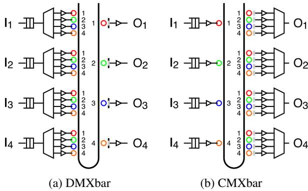
**Figure 4: Photonic 4x4 Crossbars** – Both crossbars have four inputs ( $I_{1-4}$ ), four outputs ( $O_{1-4}$ ), and four channels which are wavelength division multiplexed onto the U-shaped waveguide. Number next to each ring indicates resonant wavelength. (a) distributed mux crossbar (DMXbar) with one channel per output, (b) centralized mux crossbar (CMXbar) with one channel per input.
