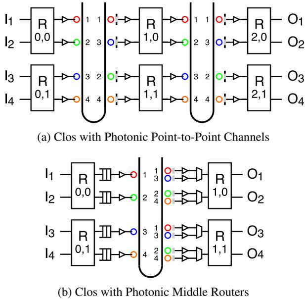
**Figure 7: Photonic 2-ary 3-stage Clos Networks** – Both networks have four inputs ( $I_{1-4}$ ), four outputs ( $O_{1-4}$ ), and six  $2 \times 2$  routers ( $R_{0-2,0-1}$ ). (a) four point-to-point photonic channels use WDM on each U-shaped waveguide. (b) the two middle routers ( $R_{1,0-1}$ ) are implemented with photonic  $2 \times 2$  CMXbars on a single U-shaped waveguide. Number next to each ring indicates resonant wavelength.
