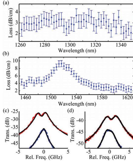
Figure 2. Propagation losses for single-mode waveguides measured near 1310nm (a) and 1550nm (b) using 4.1mm differential length structures. Measured fit transmission for drop ports of moderately-coupled (red points) and weakly-coupled (blue points) 20  $\mu$ m radius rings at 1280nm (c) and 1550nm (d).
