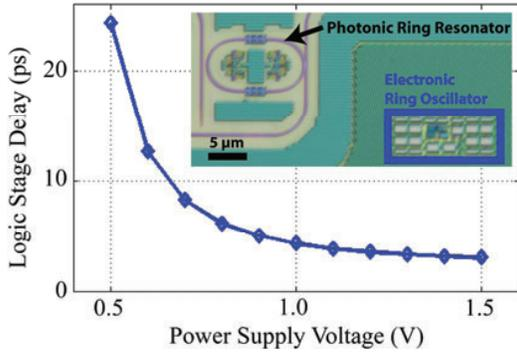
Figure 1. Stage delay of ring oscillator shown in micrograph inset.
