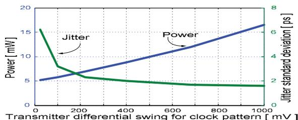
Figure 11. Power and jitter vs. output swing for a clock output pattern
