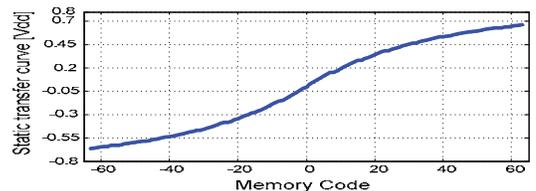
Figure 7. Static DAC transfer curve
