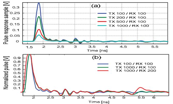
Figure 3. (a) Pulse response of Peters' 3'' channel vs.  $R_{tx}/R_{rx}$  interface resistance, (b) Normalized pulse response for Peter's 3'' channel to eliminate the scaling vs  $R_{tx}/R_{rx}$
