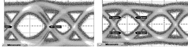
Figure 9. Joint pre-emphasis and duty-cycle correction
