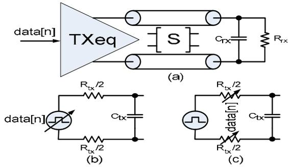
Figure 2. (a) Schematic for study of impedance modulation (b) Equivalent schematic of VM driver, (c) Equivalent schematic of RM driver voltages, as shown in Fig. 1. The power of the VM driver is given in
