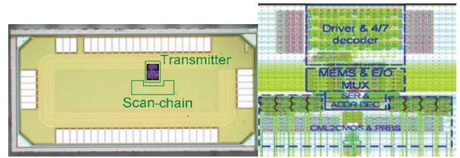
Figure 12. Die photo (1mm x 2mm) and Tx floorplan (150µm x 130µm)
