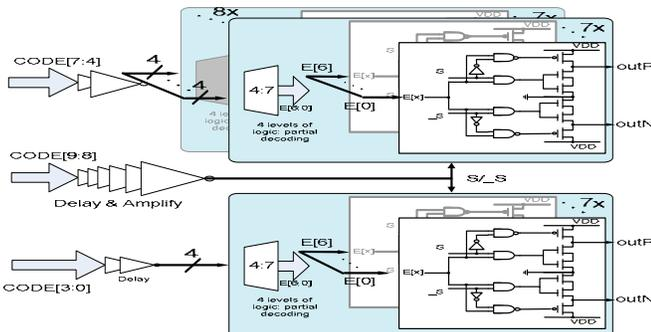
Figure 5. Simple RM output driver (asynchronous part)
