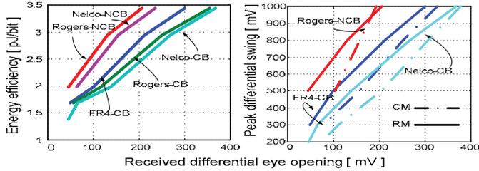
Figure 10. Energy-efficiency over various backplane channels
