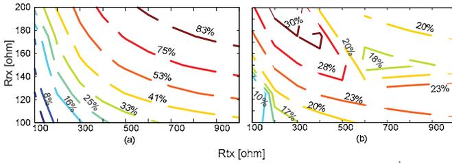
Figure 4. Relative degradation of the worst-case eye equalized by 3<sup>rd</sup> order TX filter as a function of transmit and receiver interface resistance increases dispersion and scales the response due to the resistive divider, from Fig. 2.
