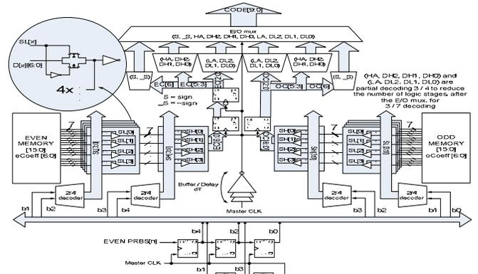
Figure 6. Decoder path of the transmitter (synchronous part)
