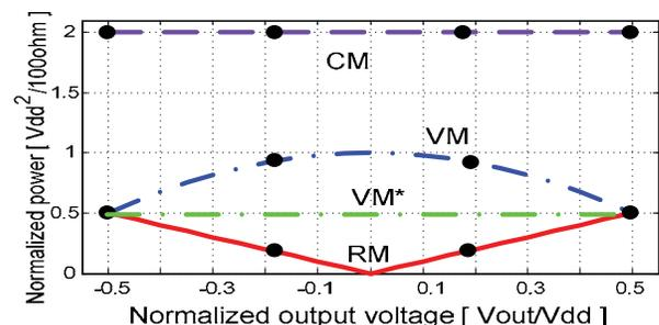
Figure 1. Normalized driver power vs. normalized output voltage
