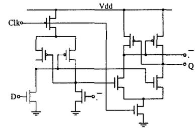
Figure 7. DSTC MS Latch
