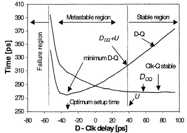
**Figure 2. StrongArm110 flip-flop, Stable, Metastable and Failure regions**
