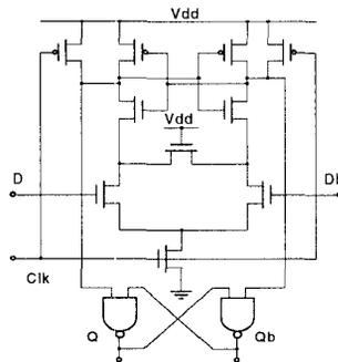
Figure 12. SArm10 Flip-Flop
