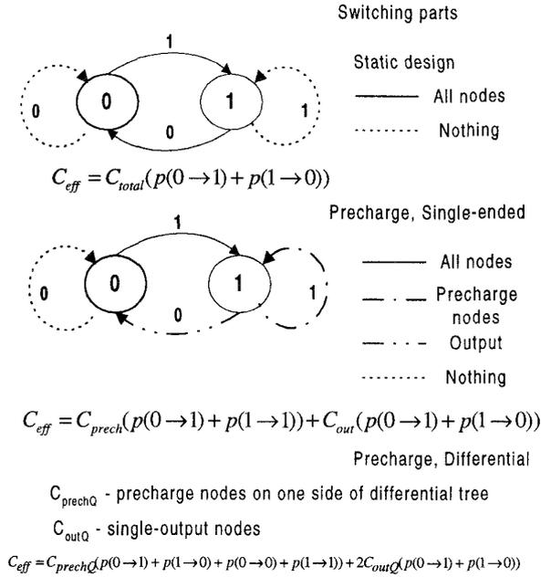
**Figure 1. Sources of internal, dynamic power consumption**
