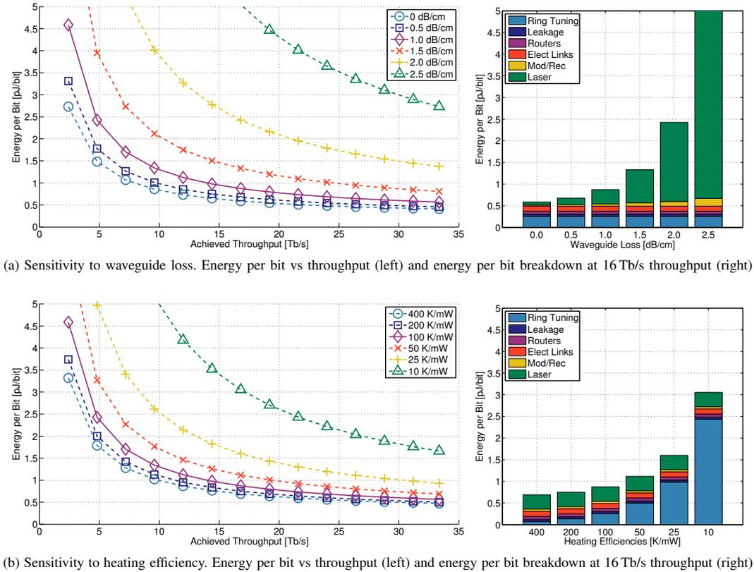
Fig. 6: Sensitivity of the photonic crosstalk network to a few select technology parameters. All plots assume the 11 nm electrical technology model.
