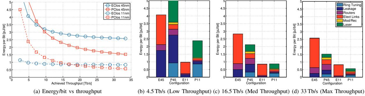
Fig. 5: Comparison of network energy per bit vs network throughput (a) and the energy per bit breakdown at various throughputs (b–d) for the electrical crosstalk (EClos) and photonic crosstalk (PClos) at both the 45nm and 11nm technology nodes. Utilization is plotted up to the point where the network saturates (defined as when the latency reaches  $3\times$  the zero-load latency).
