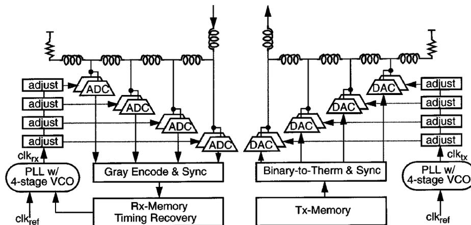
Fig. 1. Transceiver architecture (Rx on the left and Tx on the right).
