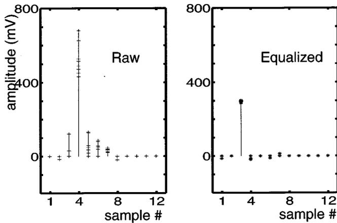
Fig. 13. Measured time-domain pulse response of the transceiver channel with inductor as sampled by the receiver both equalized and unequalized.
