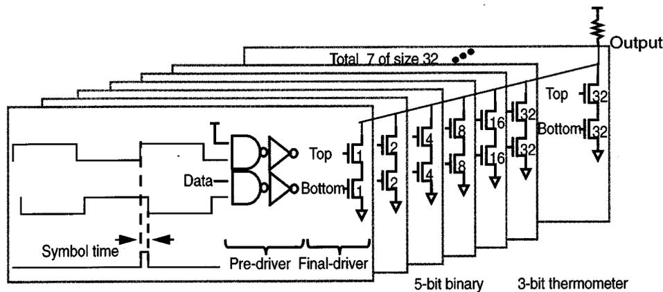
Fig. 9. D/A converter current steering architecture.
