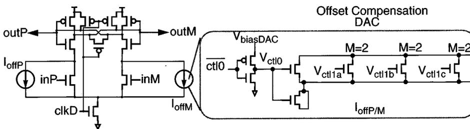
Fig. 5. Clocked offset-compensation (second-stage) latch with design of offset-current DAC.
