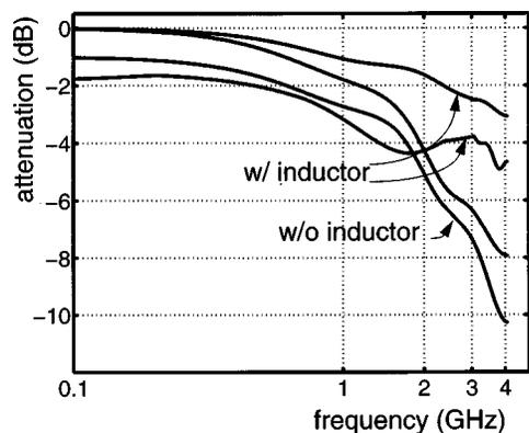
Fig. 10. Measured transmitter frequency response (envelope of all eight DACs) with and without inductor.
