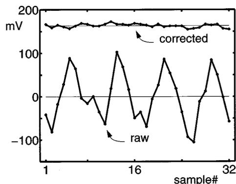
Fig. 12. DC offsets of transceiver with inductors before and after calibration.
