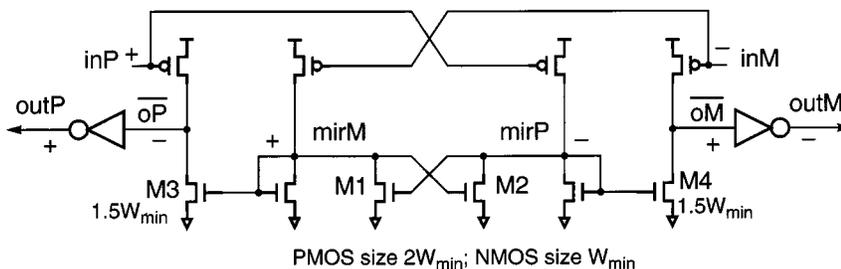
Fig. 6. Output unlocked (third-stage) latch.
