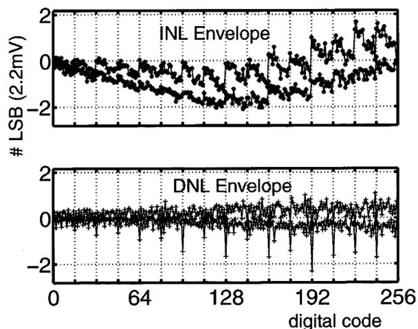
Fig. 11. Measured INL and DNL of all eight D/A converters shown as an envelope (LSB = 2.2 mV).
