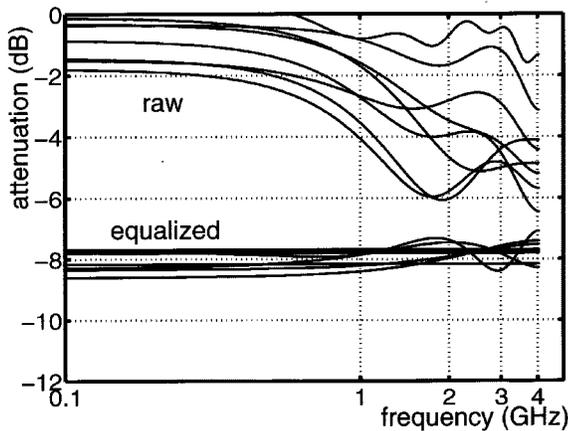
Fig. 14. Measured frequency response of the transceiver channel with inductor both equalized and unequalized.
