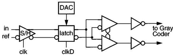
Fig. 3. Comparator block diagram.
