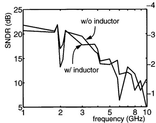
Fig. 15. Measured receiver SNDR with and without inductor.
