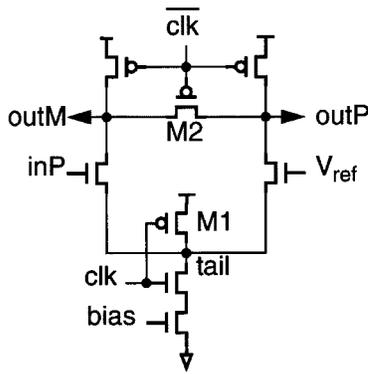
Fig. 4. Sample-hold (first-stage) amplifier design.
