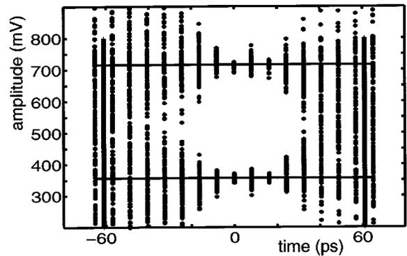
Fig. 16. Schmoop plot of binary data eye at 8 GSymbol/s.
