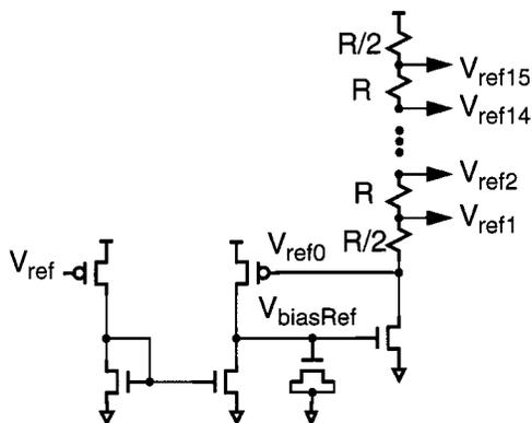
Fig. 7. Reference resistor ladder.
