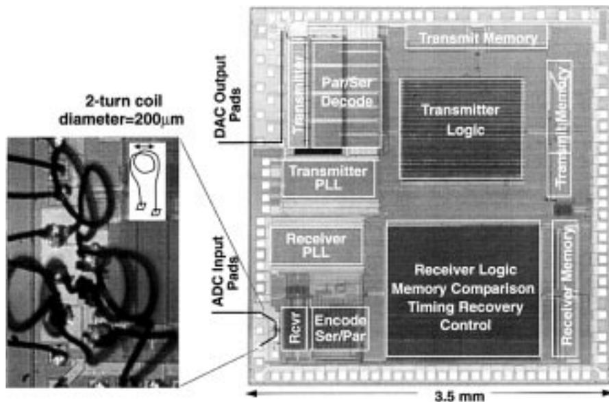
Fig. 2. Chip micrograph with the magnified image of the bonding at the ADC.
