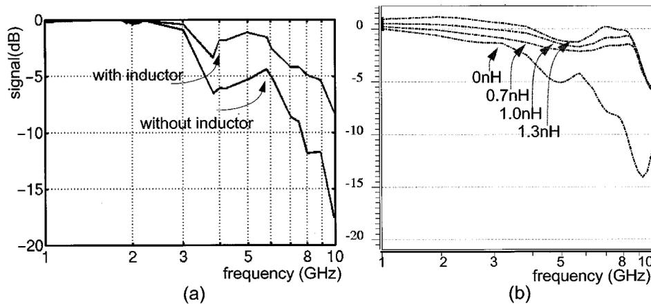
Fig. 8. Receiver bandwidth (a) measured with and without inductors and (b) simulated with various inductances.
