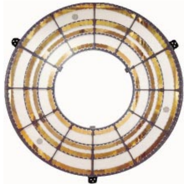
Figure 42. Photograph of the HETGS flight instrument, which consists a 1.0 meter-diameter aluminum wheel populated with hundreds of 200 nm and 400 nm-period gold x-ray transmission gratings (340 total).
