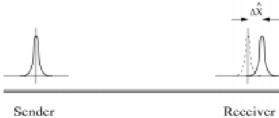
Figure 20. This figure depicts accumulated quantum uncertainty in the position of pulses in a communications system. The accumulating uncertainty in position, and thus in arrival time, of a pulse places fundamental limitations on the communication rate.
