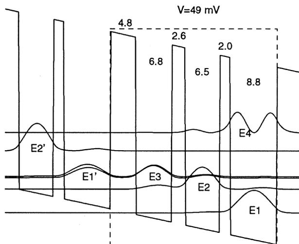
**Figure 4.** Schematic of a three-level system based on a triple quantum-well structure. The radiation transition takes place between E<sub>3</sub> and E<sub>2</sub>, and the fast LO-phonon emission keeps the level E<sub>2</sub> empty. The conduction-band profile and the square of the electron wavefunctions were calculated numerically from Schrödinger and Poisson equations.
