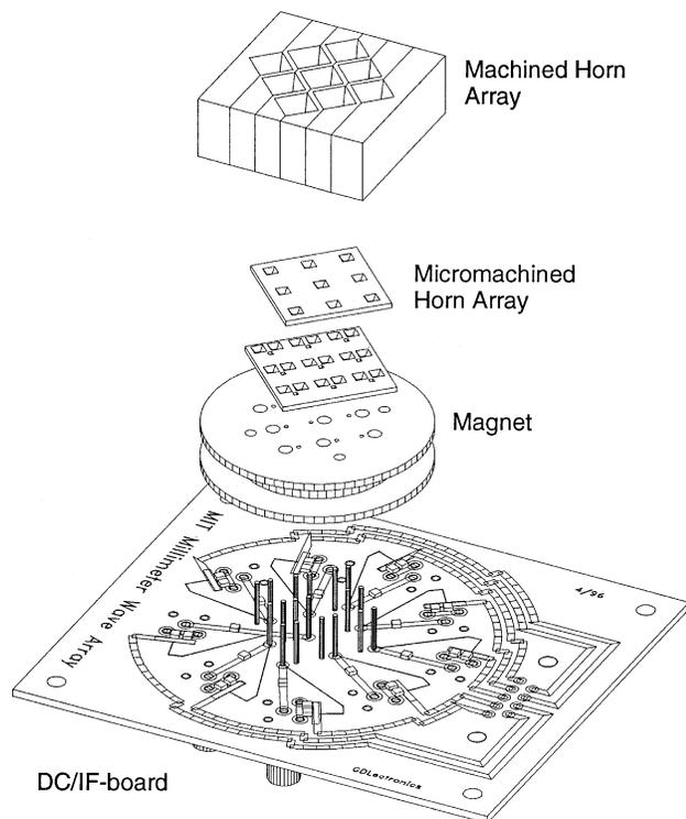
**Figure 2.** (a) Schematic of an array structure including a micromachined and machined horn array, the device wafer, and the dc and IF connection board. (b) I-V curves of seven SIS junctions in the array.
