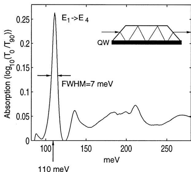
**Figure 5.** Infrared absorption measurement of a 80-module device, which was placed at room temperature. The absorption peak is due to the  $E_1 \rightarrow E_4$  intersubband transition. The measured FWHM is 7 meV, including a 4-meV instrumental linewidth. The measured intersubband transition frequency (110 meV) and dipole moment (14 Å) agreed quite well with the calculated values of 109 meV and 12 Å.
