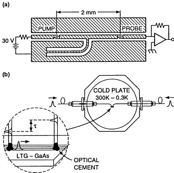
**Figure 11.** (a) Two Austin switches coupled through a coplanar transmission line. (b) Schematic of a cryostat with optical-fiber couplers that bring subpicosecond laser pulses to the cryogenic stage.
