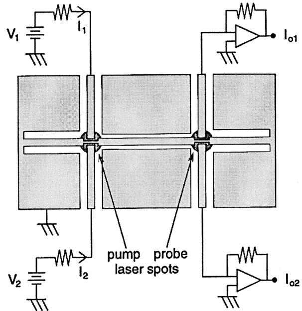
**Figure 12.** A novel coplanar waveguide structure that provides an easy integration with a three-terminal device and a compensation of misaligned optical pulses.
