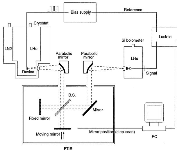
**Figure 6.** Far-infrared measurement set-up that uses an external Fourier transform spectrometer to spectrally resolve the emitted THz signals.
