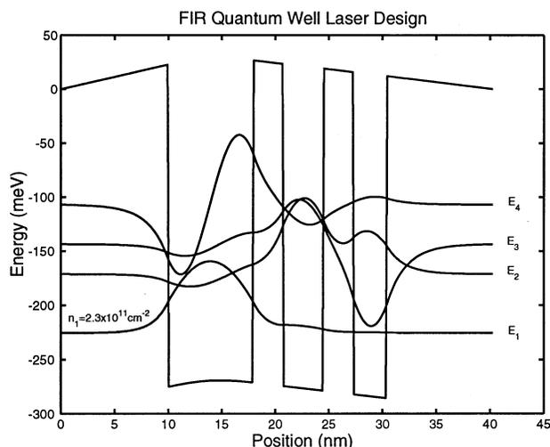
**Figure 7.** Schematic of a four-level system based on a coupled triple quantum-well structure. Electrons can be pumped from the  $E_1$  to the  $E_4$  level by a  $\text{CO}_2$  laser. They then quickly relax to the  $E_3$  level by LO-phonon scattering. Similarly, the electrons on the  $E_2$  level can be emptied quickly to  $E_1$  through LO-phonon scattering. THz emission takes place between  $E_3$  and  $E_2$ .
