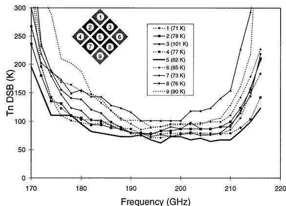
**Figure 3.** Measured DSB noise temperatures of all the nine elements in the array. The inset shows the minimum noise temperature for each element.
