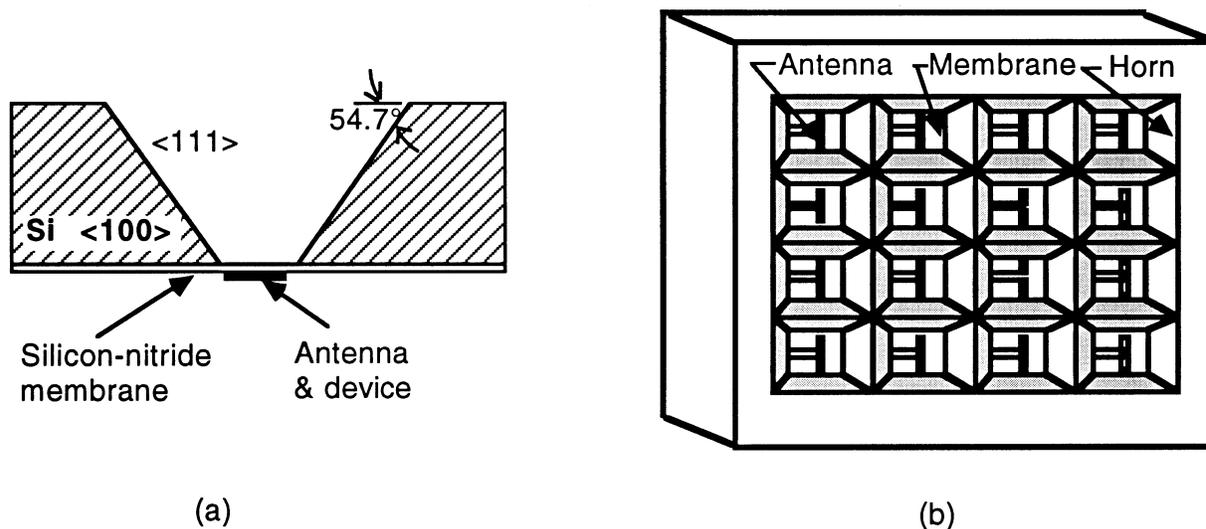
**Figure 1.** (a) Example of a micromachined horn antenna structure that is made by anisotropically etching a <100> silicon wafer. (b) Schematic of a focal-plane array on a single wafer made using micromachining.
