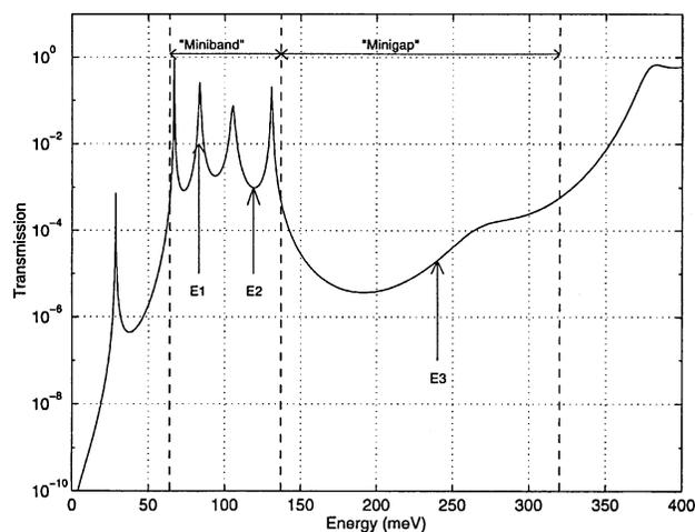
**Figure 9.** Calculated transmission coefficient of the superlattice sandwiching the core structure. The valley in the transmission corresponds to the minigap and the peaks form the miniband.
