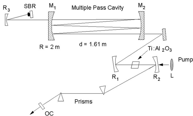
Figure 1: Ti:Al<sub>2</sub>O<sub>3</sub> laser schematic with a pair of multiple pass cavity mirrors: M1, M2, 2" diameter MPC mirrors(Spectra-Physics) with R = 2 m radius of curvature; R1, R2, 10 cm radius of curvature mirrors (Spectra-physics); L, 6.3 cm focal length pump beam focusing lens; OC, 27% 1/2" thick output coupler (Spectra-Physics); Prisms, fused silica prisms.
