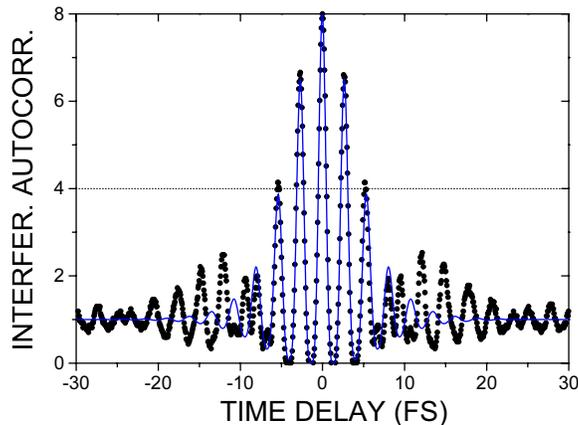
Figure 4: Measured interferometric autocorrelation (dots) of the Ti:Al<sub>2</sub>O<sub>3</sub> laser pulses. The dashed curve is a fit of sech<sup>2</sup>-function with a FWHM of 5.4 fs, and the solid curve is the calculation from the spectrum.
