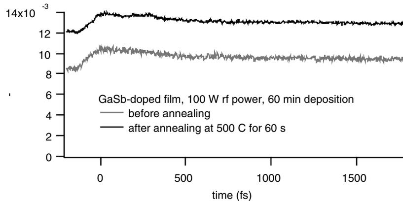
Figure 6: GaSb-doped silica films grown at 100 W for 60 min before and after rapid thermal annealing at 500°C for 60 seconds.
