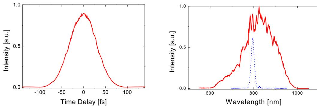
Figure 3: (a) Intensity autocorrelation trace showing a pulse duration of 44 fs assuming a  $\text{sech}^2(t)$  intensity profile, (b) Continuum generation through a 0.55 NA focusing lens into a single mode fiber (3M, FS-SC-3314); spectrum of an initial pulse (dotted line), generated continuum (solid line).
