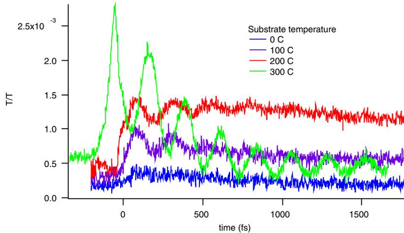
Figure 7: Coherent phonon generation in GaSb+SiO<sub>2</sub> films. Films were grown at 100 W rf power for 30 min and the substrate temperature was varied from 0°C to 300°C.
