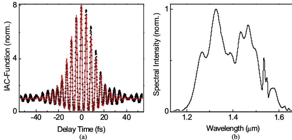
Figure 5: (a) Measured autocorrelation of the Cr:Forsterite laser output showing 14 fs pulse duration. (b) Measured laser output spectrum. These pulse durations are made possible using intracavity dispersion management with double chirped mirrors (DCM's). The pulse duration is the shortest ever generated from a Cr:Forsterite laser.
