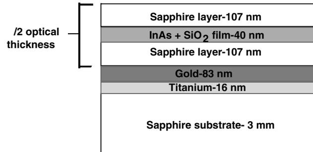
Figure 8: Design of a reflective saturable absorber device with sapphire spacer layers on a gold mirror.
