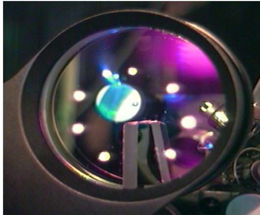
Figure 2: Photograph of an MPC mirror with 8 bounces per mirror used in a 5 MHz Ti:Al<sub>2</sub>O<sub>3</sub> laser with a separation of 161 cm between two MPC mirrors.
