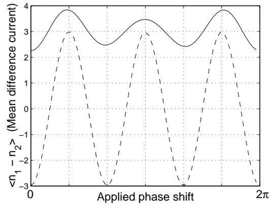
Figure 2: Numerical results: fringes with enhanced phase sensitivity are calculated for a photon-number state and a coherent state. The number uncertainty of the coherent state reduces the contrast of the fringes, but leaves the basic physics of photon tunneling intact.
