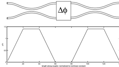
Figure 1: Conceptual sketch of nonlinear coupler with adiabatic variation of linear coupling.
