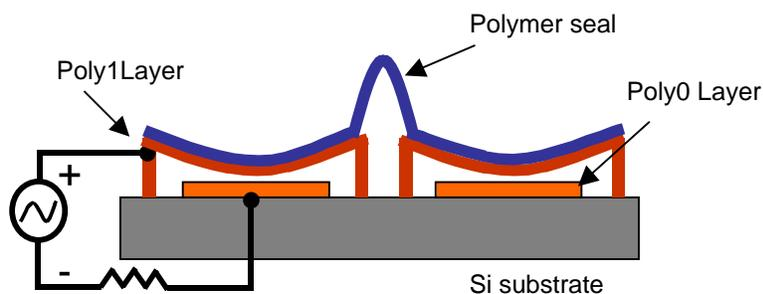
Figure 3.2-1. Surface Micro-machined Actuator with Polysilicon Membrane.
