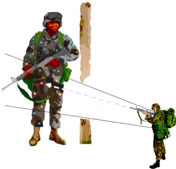
*Figure 4.2-1. Depicts envisioned usage of bodyworn haptic stimulators in combat simulation. Self-contained pods distributed about the surface of the user signal exposure, contact, and impact, based on their position relative to objects in the virtual world. Signals can be mechanical (e.g., vibration) or electrical (e.g., electrocutaneous stimulation).*
