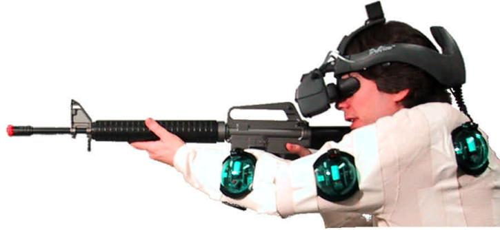
*Figure 4.2-2. Depicts usage of bodyworn haptic stimulators in context of immersive virtual environment presentation. Weapon is instrumented with infrared laser tracking and wireless communication of trigger state.*
