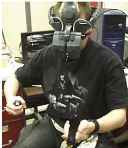
*Figure 4.3-1. World In Miniature simulation in use with head-mounted display and handheld operator interfaces to control and interact with the display.*
