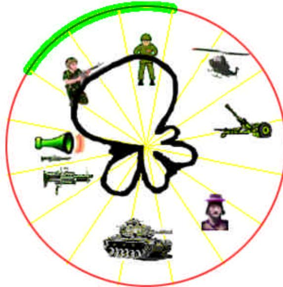
*Figure 6.1-1. Polar plot depicting sensitivity of microphone array at one moment in time during complex battle audio scene. The system in this case is attempting to preserve the upper left sectors while attenuating the remaining sectors.*
