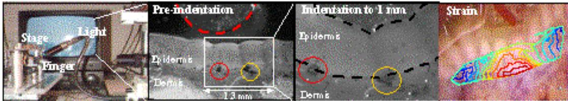
Figure 3.1-1. A video microscopy system (left image) provides high resolution images of skin. A cylindrical indenter loads a cadaver finger pad, while the tissue is viewed in cross section (middle 2 images). Strains around mechanoreceptors are estimated from displacements of markers on the tissue (right image).
