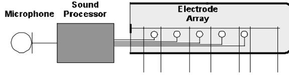
in the cochlea and connected to a sound processor. The sound processor (typically DSP-based) is programmed to translate the output of the microphone into electric stimuli delivered to the implanted electrodes. The number of processing and stimulation channels range from 4 to 24.
