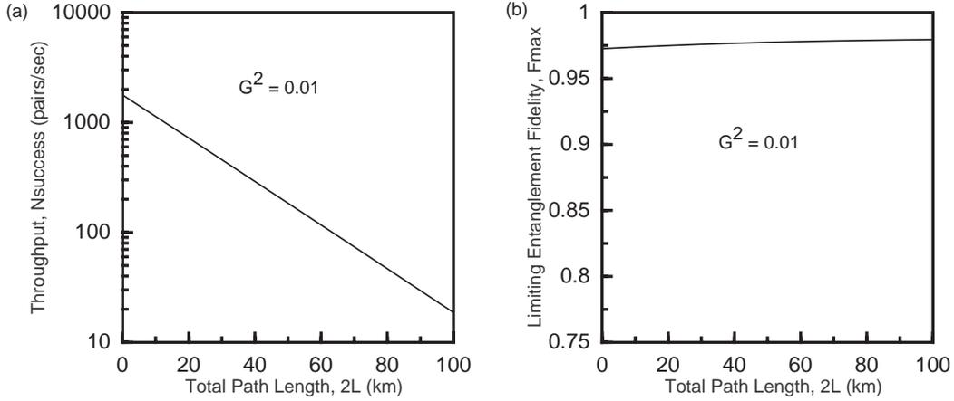
Figure 5. Figures of merit for Fig. 1 configuration. Left (a), throughput,  $N_{\text{success}}$ , vs. total path length,  $2L$ . Right (b), limiting entanglement fidelity,  $F_{\text{max}}$ , vs. total path length,  $2L$ .
