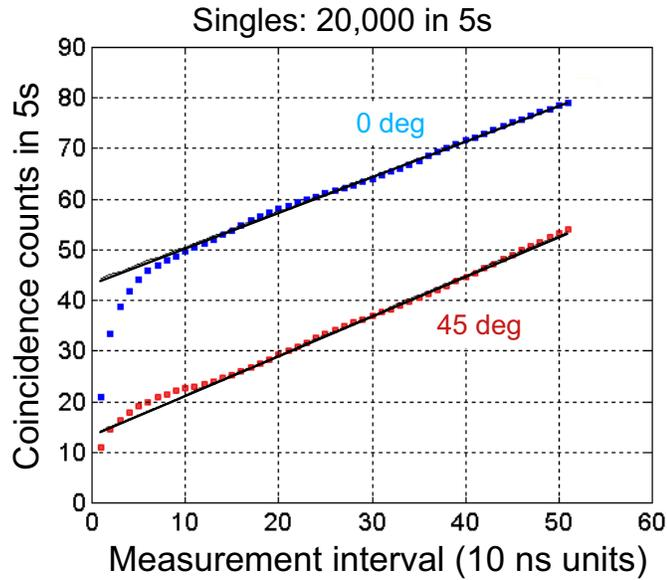
Figure 7. Coincidence counts vs. measurement time bins for (a) 0° polarization rotation and (b) 45° polarization rotation.
