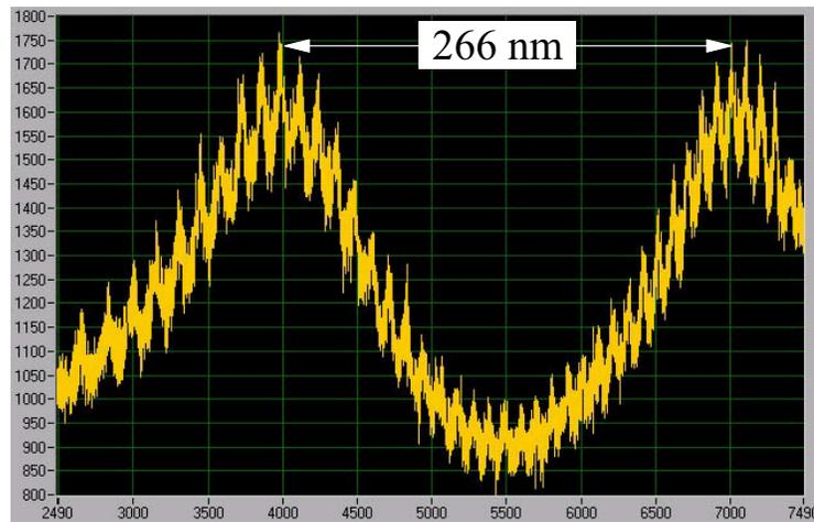
Figure 6. Trace of detected singles count as cavity length is swept.
