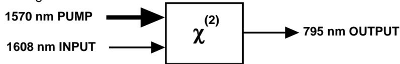
Figure 3. Schematic of quantum frequency conversion: a strong pump beam at 1570 nm converts a qubit photon received at 1608 nm (in the low-loss fiber transmission window) to a qubit photon at the 795 nm wavelength of the  $^{87}\text{Rb}$  quantum memory.
