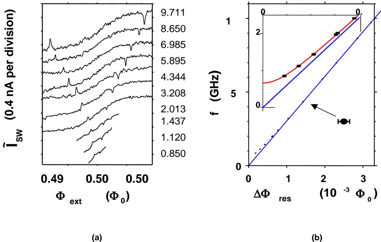
**FIGURE 2.** (a) The circulating current as inferred from the dc SQUID measurements for various applied microwave frequencies. The curves are offset for clarity. (b) Half the distance in  $\Phi_{\text{ext}}$  measured between the resonant peaks and the dips at different frequencies  $f$ . The inset shows the low frequency data points. The blue line is a linear fit through the high frequency points and zero. The red line is a fit of the quantum theory.
