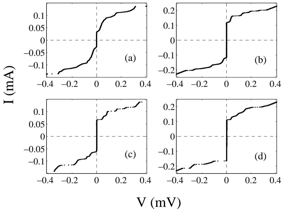
**FIGURE 8.** Sample IV curves for the four measured rings. Rings (a), (b), and (c) have symmetric IV's as the current is swept in the positive and negative direction. The measurements correspond to  $M=1$ . Ring (d) is the ratchet ring as can be seen from the difference in the depinning current in the positive and negative direction.
