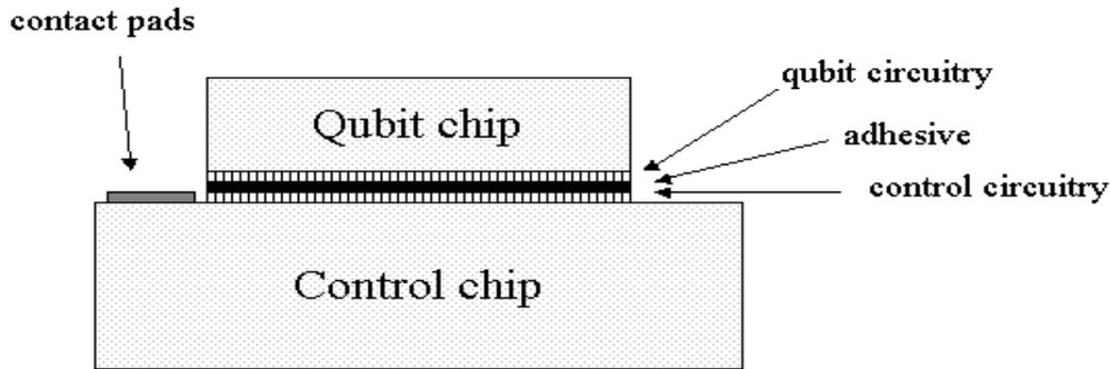
**FIGURE 3.** Cross section of a packaged chip. For our initial experiment, the “qubit” chip contained the transformer loop while the “control chip” included the control line and dc SQUID, coupled together via the transformer loop.
