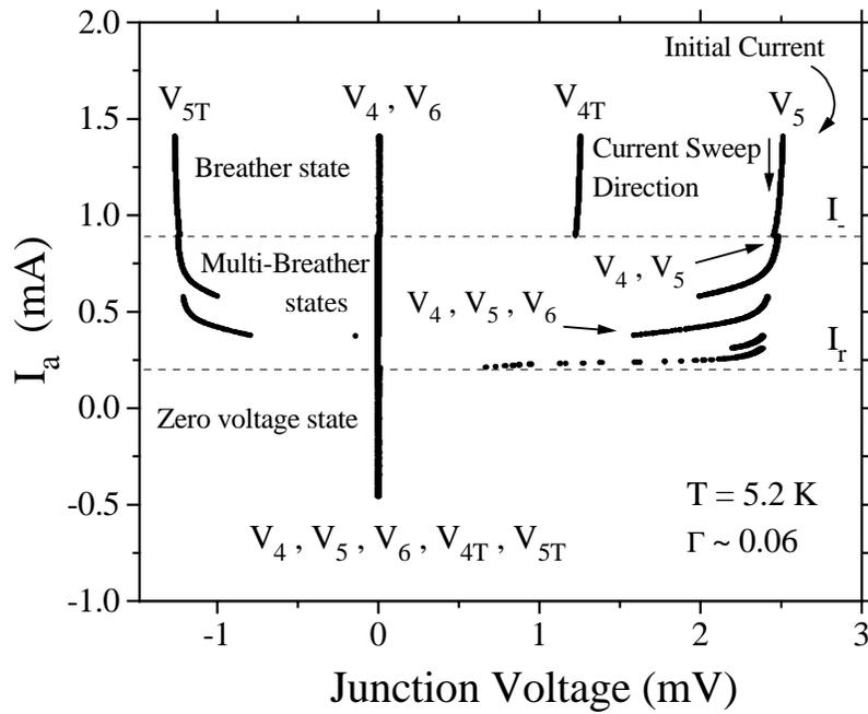
**FIGURE 10.** Measured time-averaged voltages of five junctions in the center of an array as the applied current is decreased. We have biased the ladder at 1.4 mA and excited a breather. Then the applied current is decreased.
