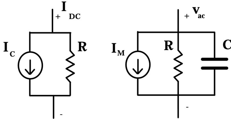
**FIGURE 5.** Equivalent circuit for a Josephson junction in a voltage state and with a single harmonic. Non-linearity is captured by  $I_M$  which is a mixing current that describes the interaction between the rotating Josephson phase and its first harmonic.
