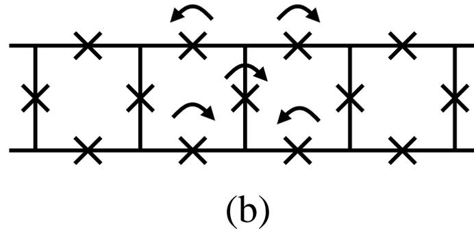
**FIGURE 9.** Schematic picture of breather solutions in ladder array: type A (a) and type B (b) breathers. Arrows are associated with rotating junctions.
