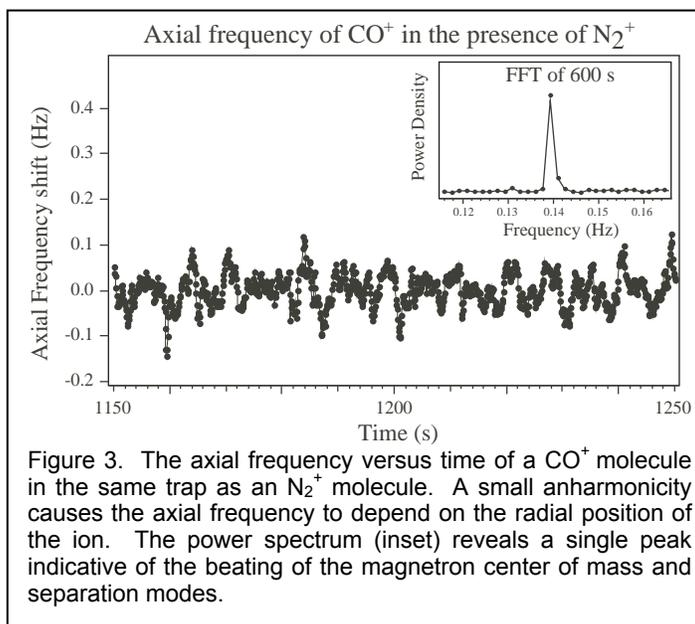
Figure 3. The axial frequency versus time of a CO<sup>+</sup> molecule in the same trap as an N<sub>2</sub><sup>+</sup> molecule. A small anharmonicity causes the axial frequency to depend on the radial position of the ion. The power spectrum (inset) reveals a single peak indicative of the beating of the magnetron center of mass and separation modes.
