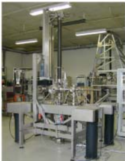
Fig.16 (a). Low temperature, high vacuum scanning probe microscope. Temperature range 5.5K-300K. (b). A 455 \times 455 \text{ nm}^2 STM scan taken at room temperature and high-vacuum showing monoatomic gold steps on a gold sample. Each step is 0.27nm in height.
