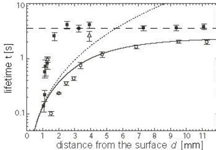
**Fig. 4.** Trap lifetime as a function of distance from a dielectric (solid squares) and metal (open circles) surface, for a temperature of 1 $\mu$ K. The dotted line is the calculated lifetime above the metal due to thermal magnetic fields only, the solid line includes the distance-independent one-body lifetime.
