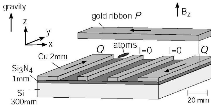
**Fig. 3.** Microfabricated chip. The outer Cu wires (Q) generate a 2D quadrupole field in the  $xz$  plane, the ribbon (P) in combination with an external field gradient creates the confinement along the  $y$  direction.
