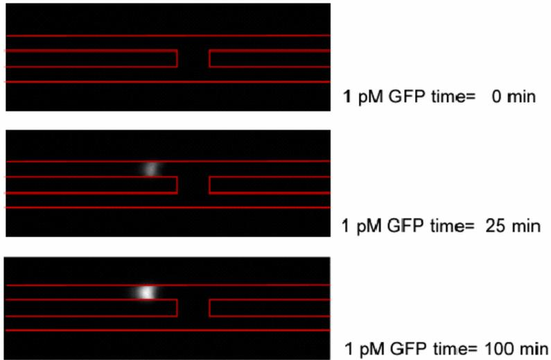
**Figure. 1.** Pre-concentration phenomena for 100 minutes, starting from highly diluted 33pM (10-12M) GFP solution. The detection condition barely detects the 33 $\mu$ M GFP concentration, which means at 25 min or later, the concentration of the plug exceeds 1 $\mu$ M. Voltage applied across top-down channel is 10 volts, while 4 volts along the top channel (pictures were taken by CCD camera with 1 sec exposure)
