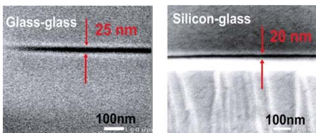
**Figure 1:** Cross-sectional SEM images of the glass-glass channel with a depth of 25 nm (A) and silicon-glass channel with a depth of 20 nm (B).
