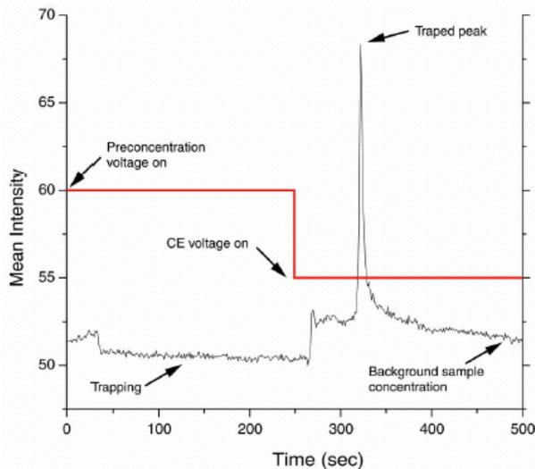
**Figure. 2.** Picture showing the electrokinetic capture/release profiles. After 250 sec, the waster channel was floated to perform an EOF- driven CE in the top channel. Shown between 300 and 350 sec is the releasing of captured proteins.
