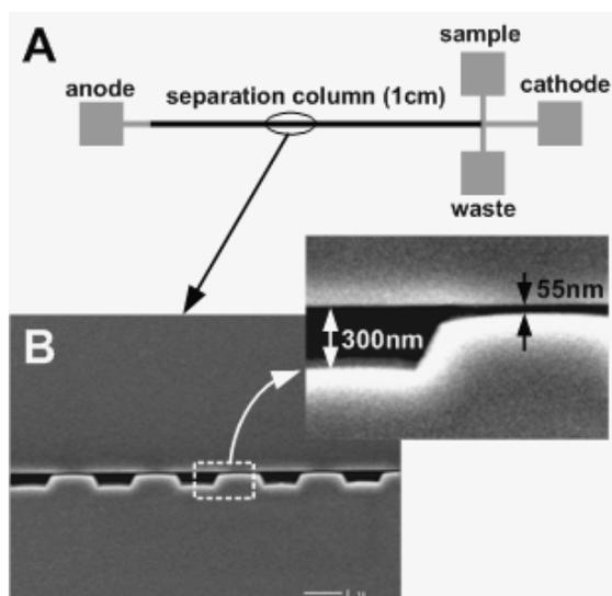
**Fig. 1. (A)** Layout of the nanofilter array chip. The device includes four buffer access holes (anode, cathode, sample and waste), a 1cm separation column (a periodic array of nanofilters) and a T-Shaped injector. **(B)** SEM images of the cross-section of a periodic nanofilter array along the separation channel. The nanofilter consists of a thin region ( $d_s=55\text{nm}$ ) and a thick region ( $d_t=300\text{nm}$ ) of equal lengths. The period of one nanofilter is  $L$  ( $L=2\mu\text{m}$ ).
