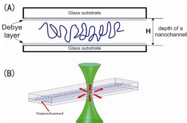
**Figure 2:** (A) Schematic diagram of a single, large DNA molecule confined to a slit glass nanochannel with a depth of  $H$ . (B) Schematic diagram of detecting single, small molecules by two-photo FCS in a slit nanochannel with vertical confinement.
