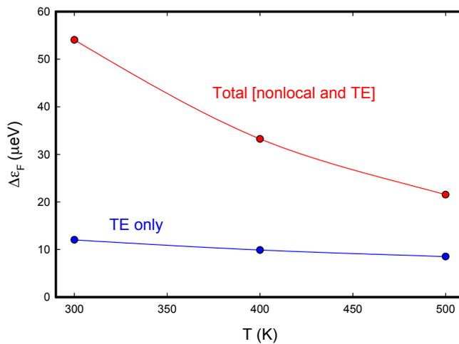
**Figure 4:** Reduction of nonlocal enhancement as a function of junction temperature for a smoothed triangular electrostatic potential profile (with small thermal gradient) due to a reduction of the scattering length.
