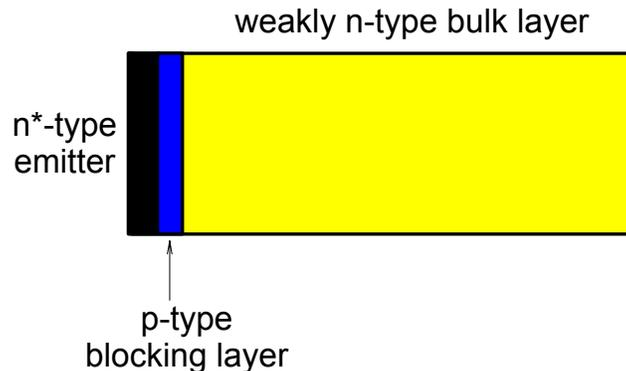
**Figure 1:** Schematic of an n\*pn-type thermal diode.
