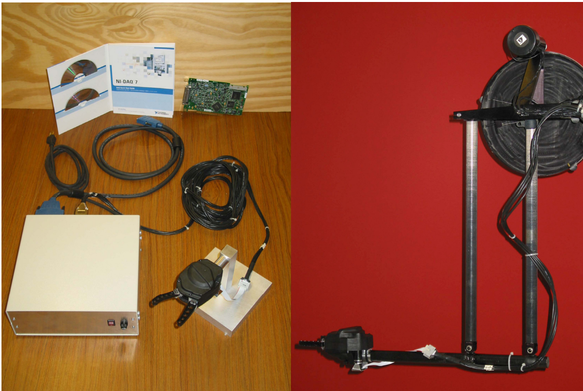
Figure 4.3-2 Gripper system (left) and gripper mounted on 3DoF phantom arm (right)
