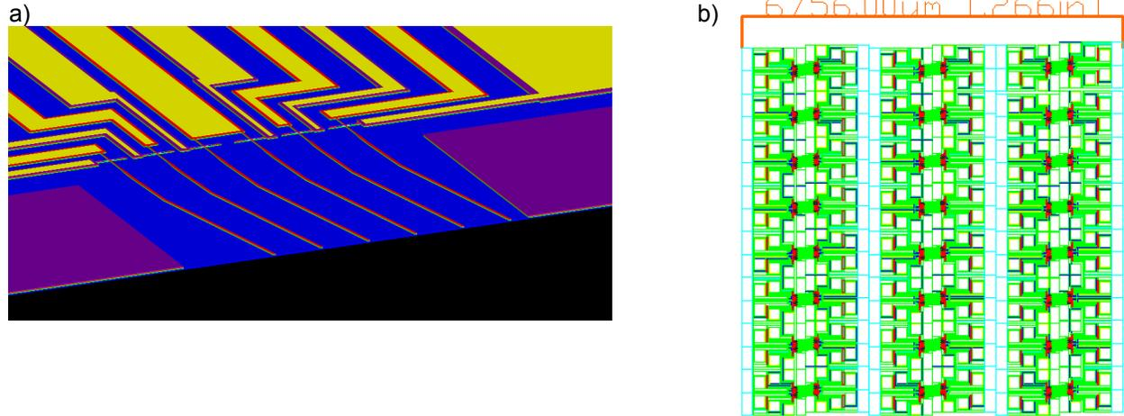
**Figure 2.** (a) Schematic of an array of 6 lasers within a 200µm field. The output waveguide is 164µm long and is angled 11° with respect to the facet. (b) Die measuring ~ 1/4" by 1/4" contains 280 different lasers. Contacts are distributed to allow easy testing.
