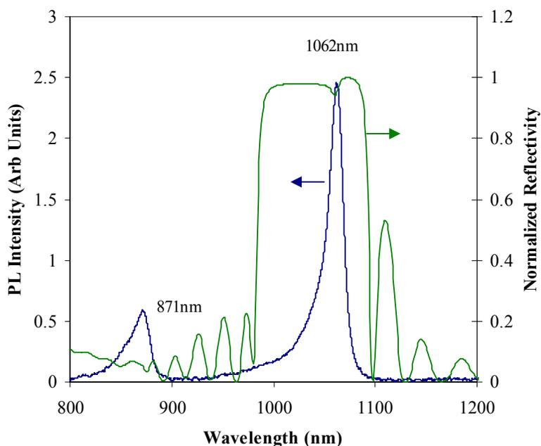
**Figure 1.** The reflectivity and photoluminescence of a InGaAs/GaAs absorber on a AlGaAs/GaAs distributed Bragg reflector.
