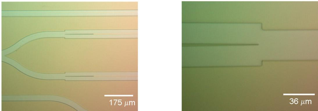
**Figure 2.** a) A photograph of the beginning of the second generation Mach Zehnder interferometer. b) A magnified view of the tip of the active waveguide prior to the definition of the lower passive waveguide.
