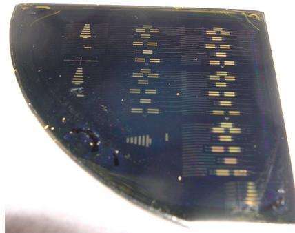
**Figure 1.** A photograph of the generation 1 fabricated dies on a quarter of a 2" InP wafer.
