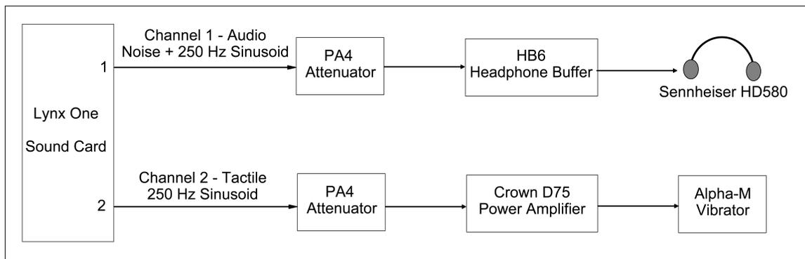
FIG 9: Block Diagram for Delivery of Auditory and Tactile Stimuli.
