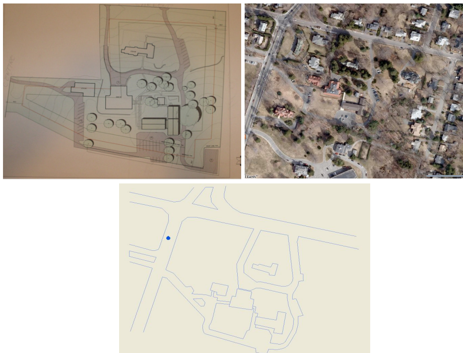
Figure 5.1-2 (a) Blueprint of the Carroll Center for the Blind campus (b) map of the campus from maps.live.com (c) a preliminary VE of the campus constructed from the above two maps
