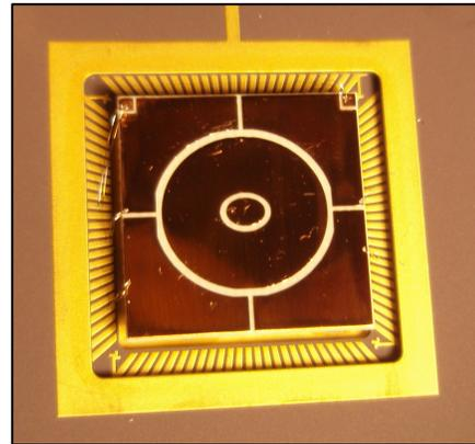
Our long-term goal is demonstrating a simple quantum simulation with three or more ions, coupled by their Coulomb interaction, modeling a Bose-Hubbard Hamiltonian, based on theory by Porras and Cirac, and taking advantage of the new surface-electrode trap geometry we have been developing. This will require sideband cooling to the motional ground state with high fidelity, traps with very long motional coherence times, and a high degree of coherent control.
